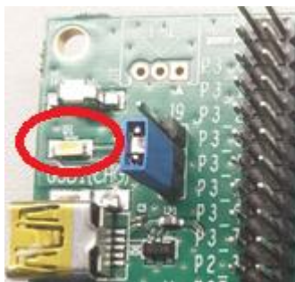
Figure 1: LED D1 on Pro DK DA1468x
