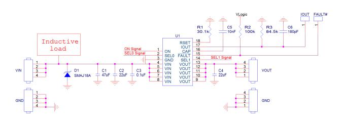
Figure 1. Transient Protection of High Voltage GreenFET using TVS
