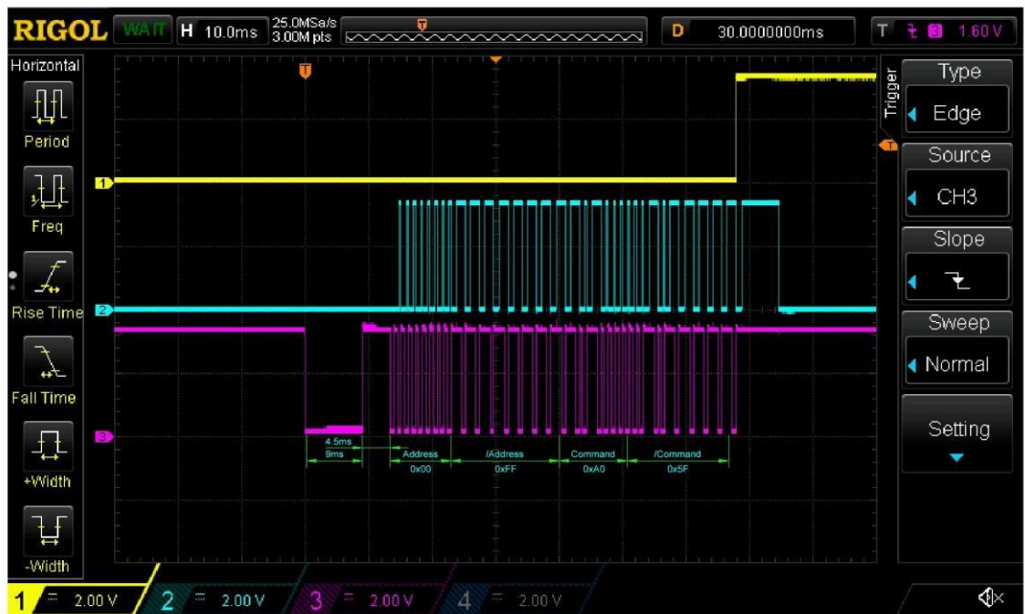
Figure 6. IR Receiver Bit Sequence
