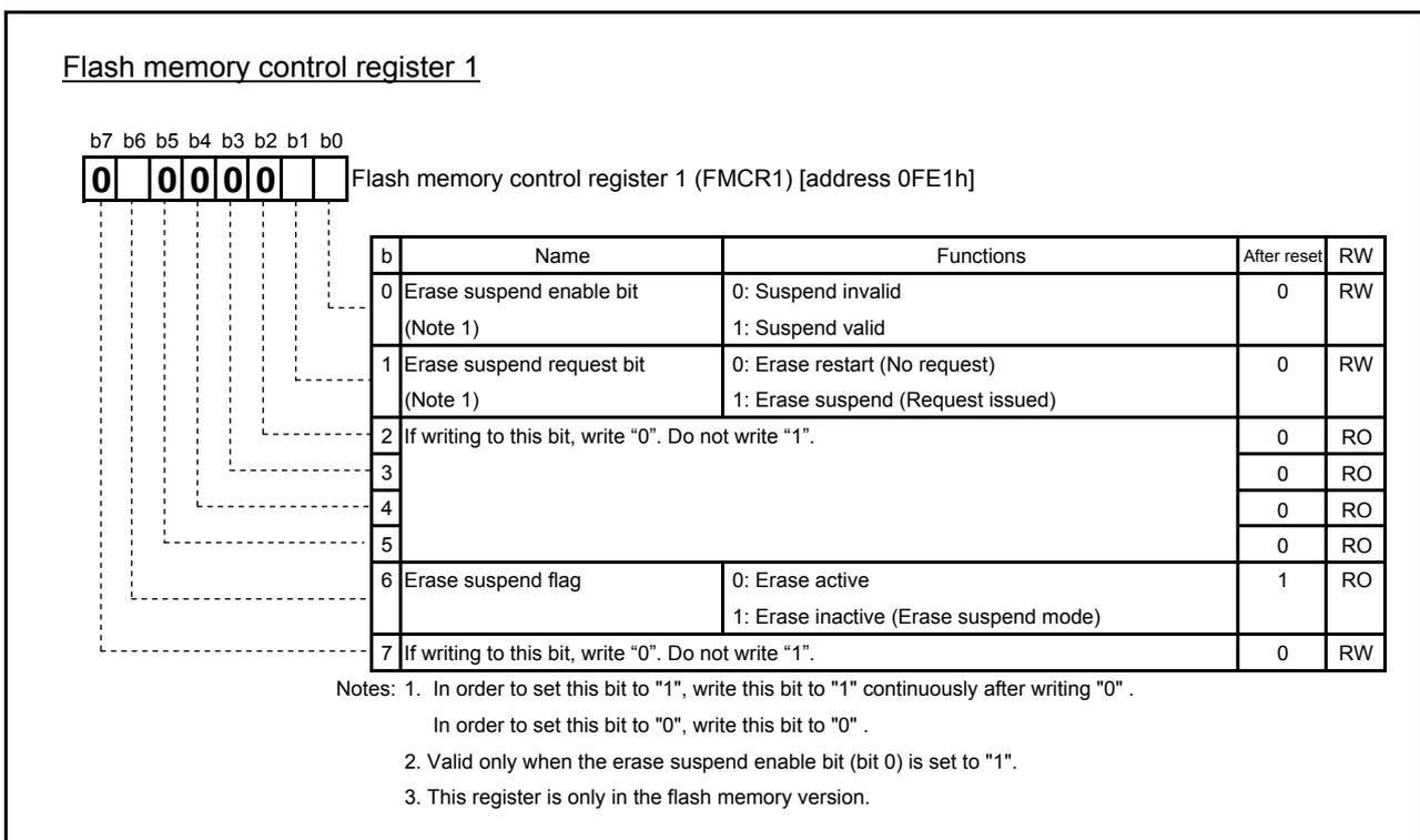
Fig.4.47 Structure of Flash memory control register 1
