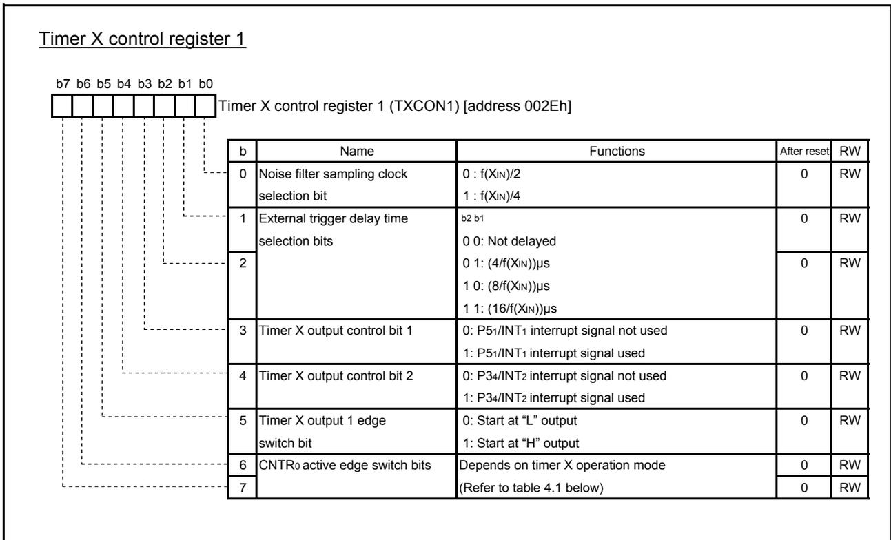
Fig. 4.34 Structure of Timer X control register 1
