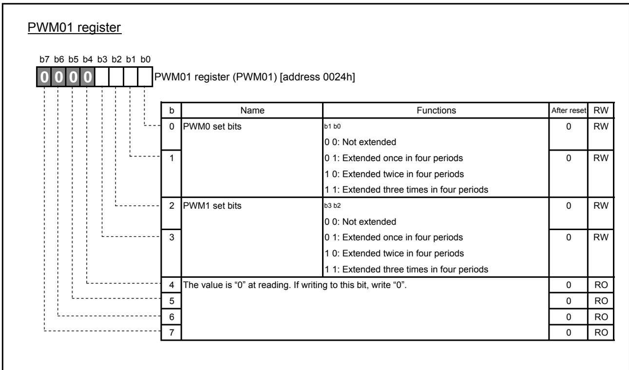
Fig. 4.25 Structure of PWM01 register
