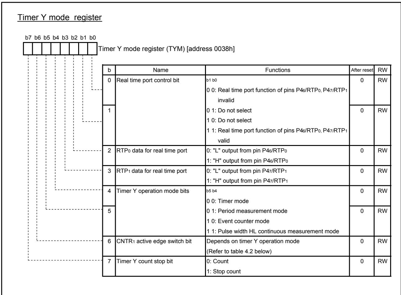
Fig. 4.38 Structure of timer Y mode register
