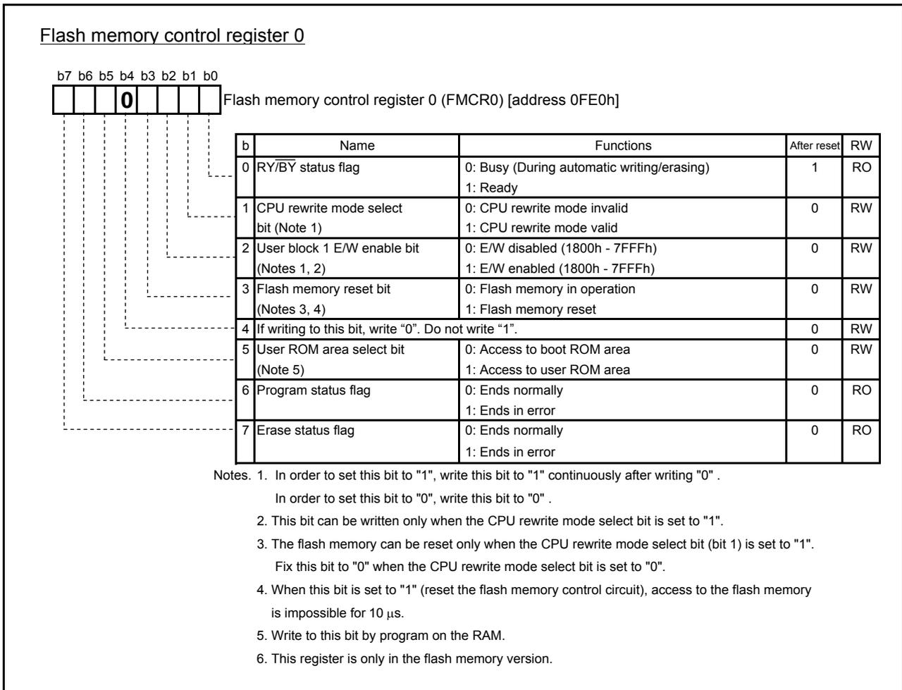
Fig.4.46 Structure of Flash memory control register 0
