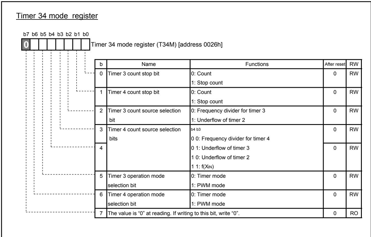
Fig. 4.27 Structure of Timer 34 mode register
