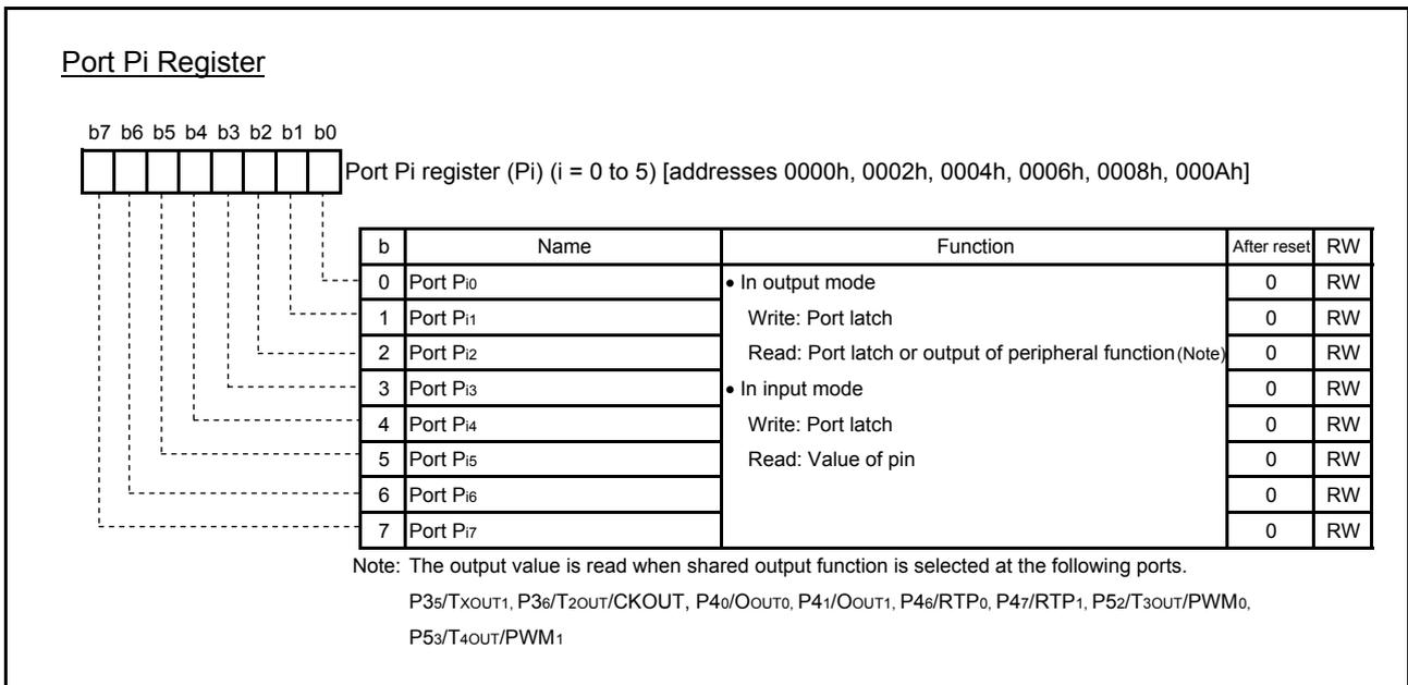
Fig. 4.1 Structure of Port Pi register (i = 0 to 5)
