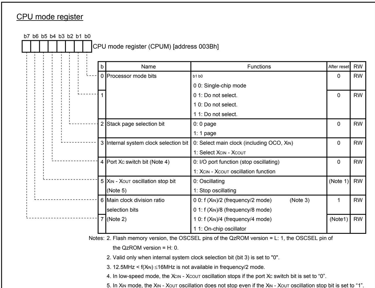
Fig. 4.41 Structure of CPU mode register
