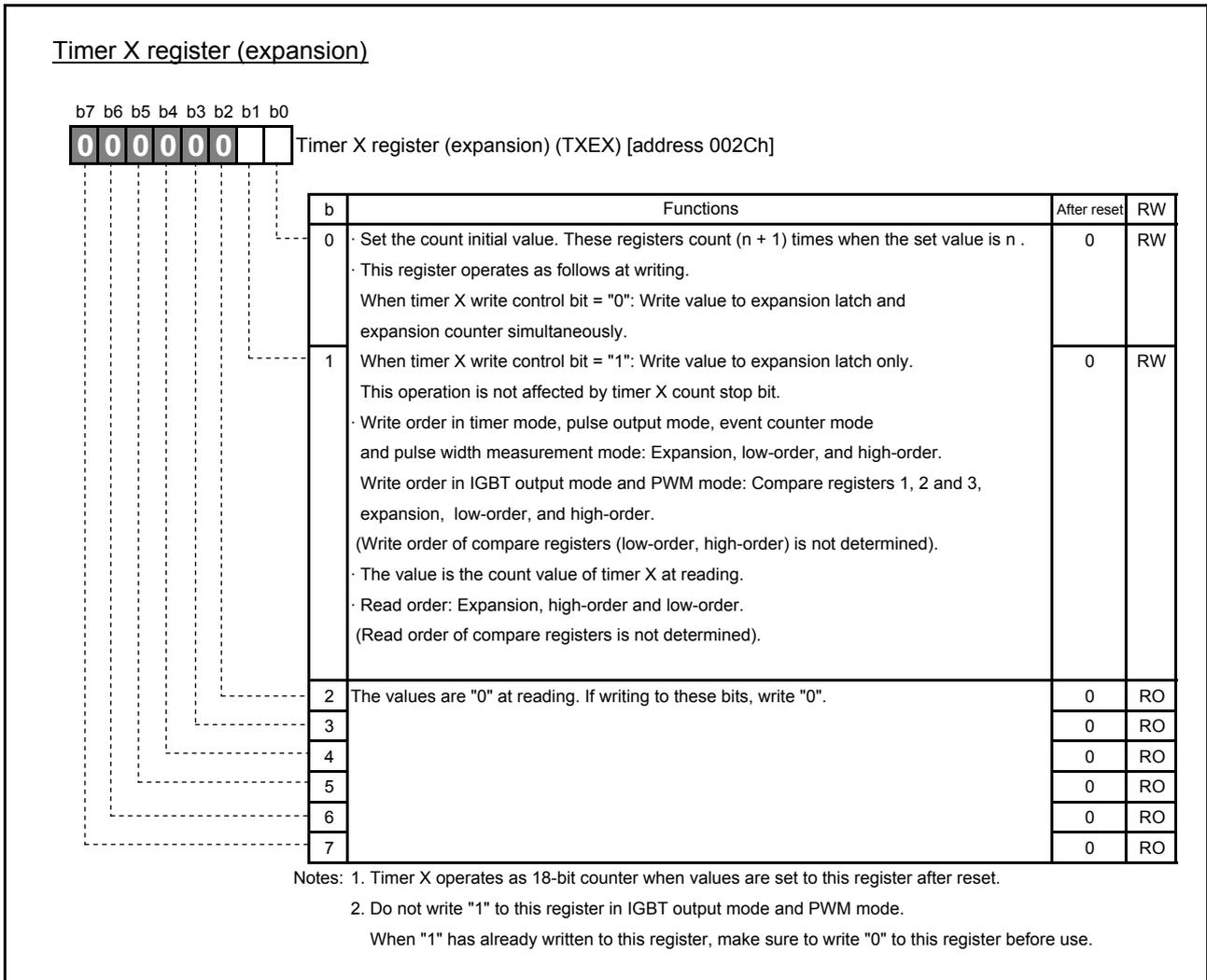
Fig. 4.32 Structure of Timer X register (expansion)
