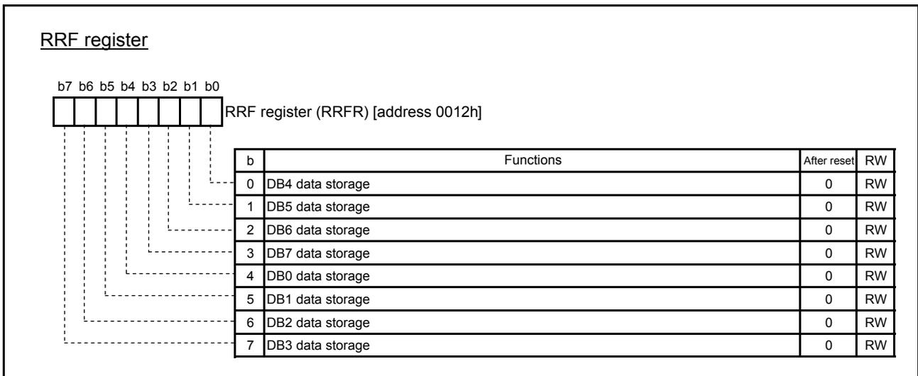
Fig. 4.7 Structure of RRF register
