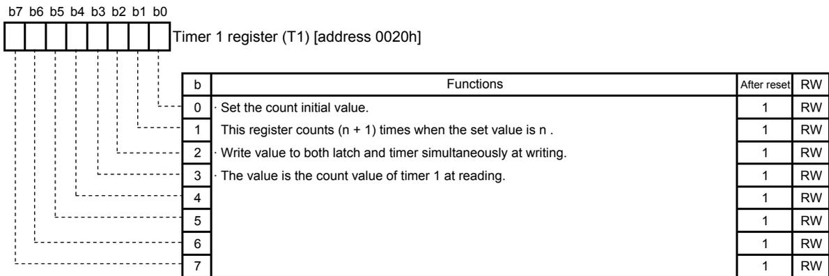
Note: This register is used to generate waiting time After reset and exiting from stop mode.
