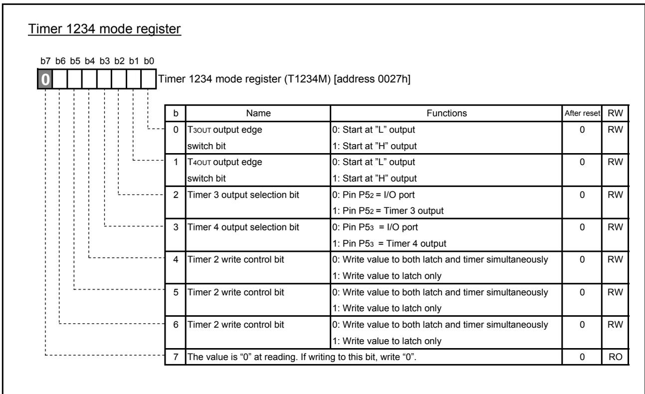
Fig. 4.28 Structure of Timer 1234 mode register
