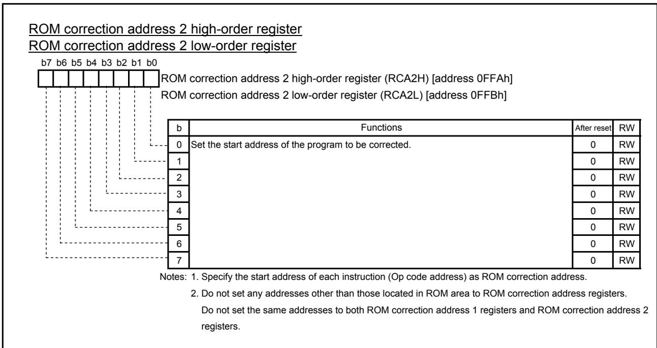
Fig. 4.57 Structure of ROM correction address 2 high-order register and ROM correction address 2 low-order register
