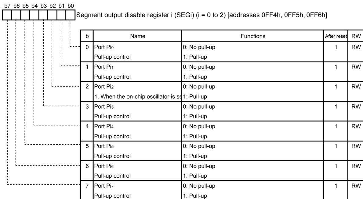
Note: When VL pin input selection bit (bit 5 at LCD power control register (address 0014h)) is set to "1", settings of P2<sub>6</sub> and P2<sub>7</sub> become invalid.
