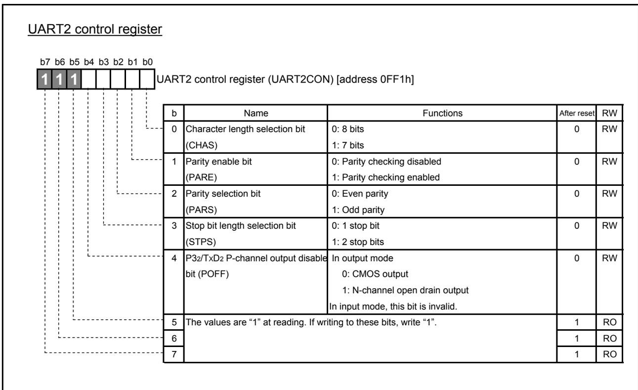
Fig. 4.48 Structure of UART2 control register
