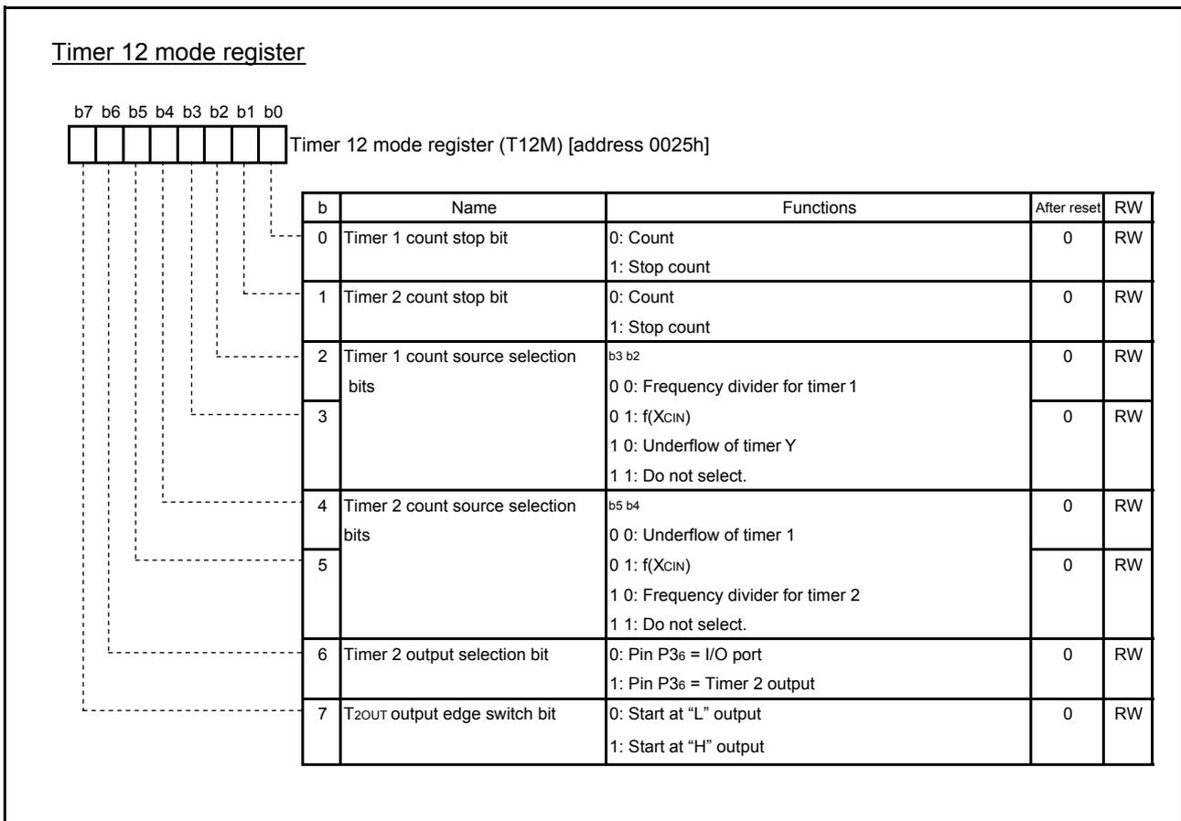
Fig. 4.26 Structure of Timer 12 mode register
