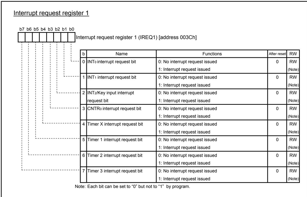
Fig. 4.42 Structure of Interrupt request register 1
