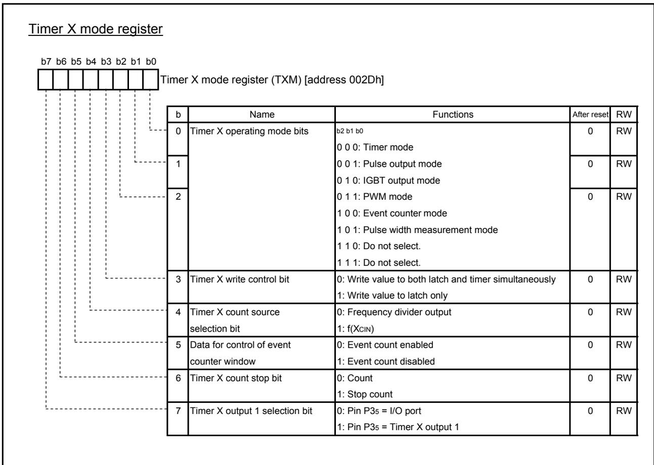
Fig. 4.33 Structure of Timer X mode register
