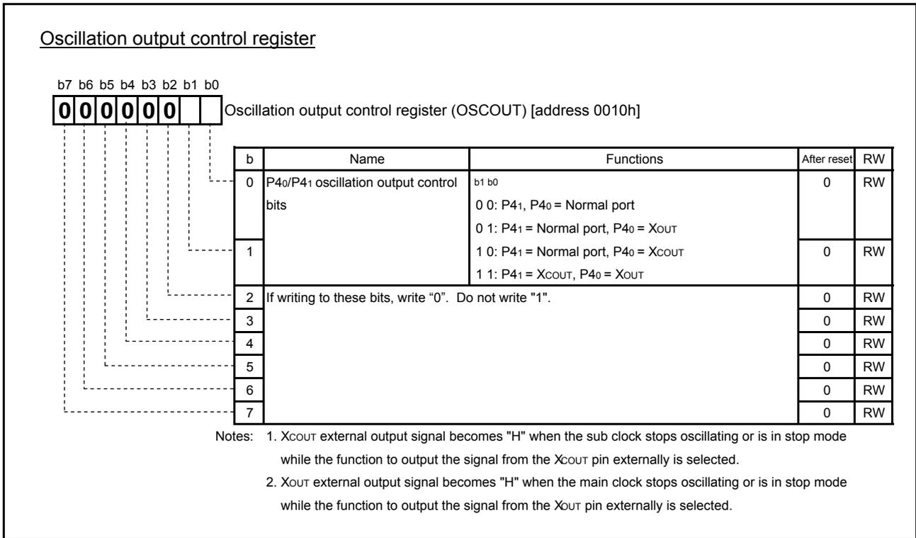
Fig. 4.5 Structure of oscillation output control register
