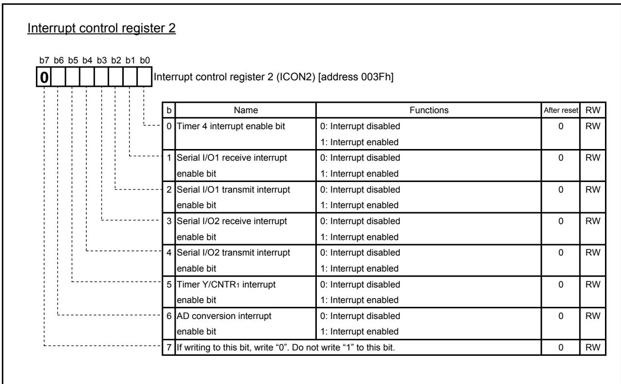
Fig. 4.45 Structure of Interrupt control register 2
