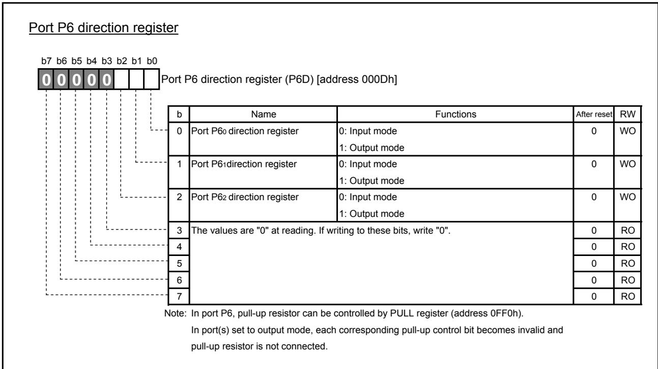
Fig. 4.4 Structure of Port P6 direction register
