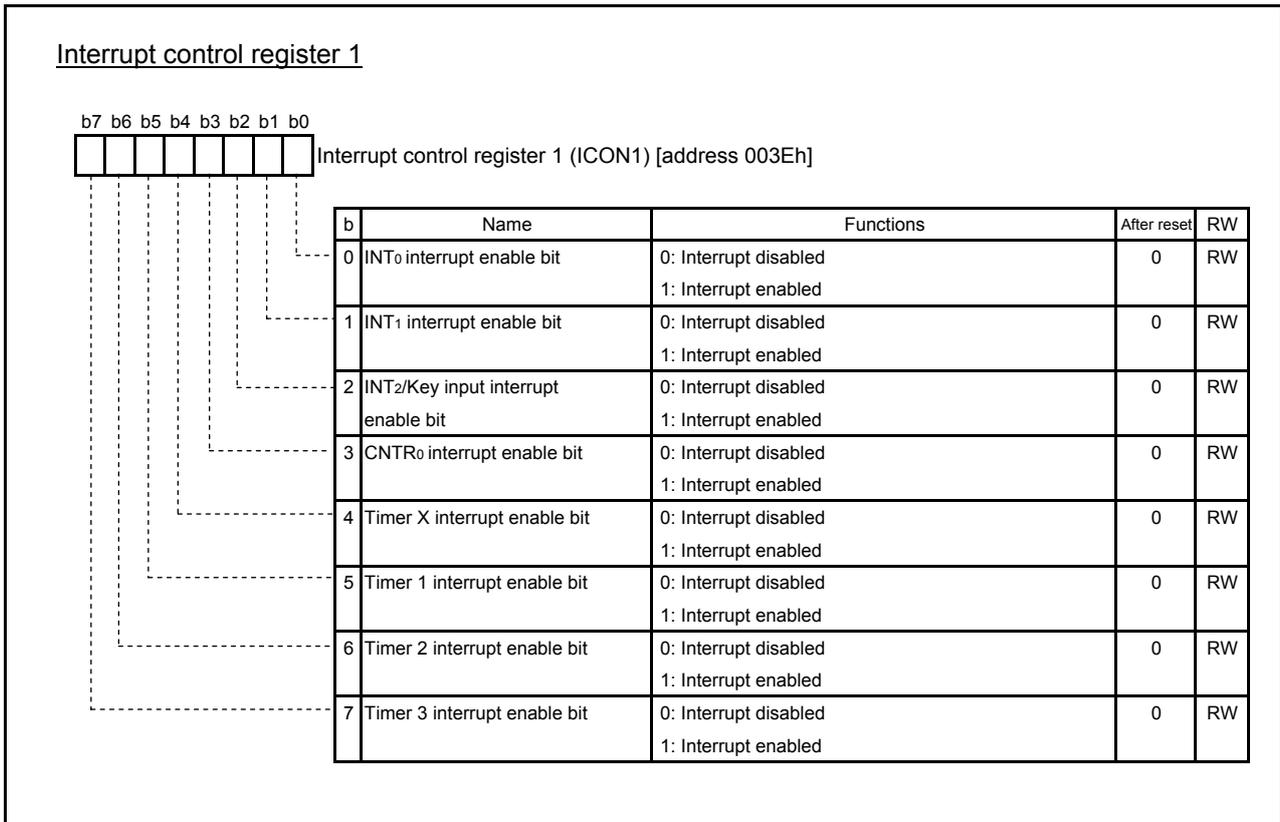
Fig. 4.44 Structure of Interrupt control register 1
