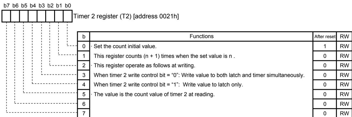
Notes: 1. This register is used to generate waiting time at reset and exiting from stop mode.
