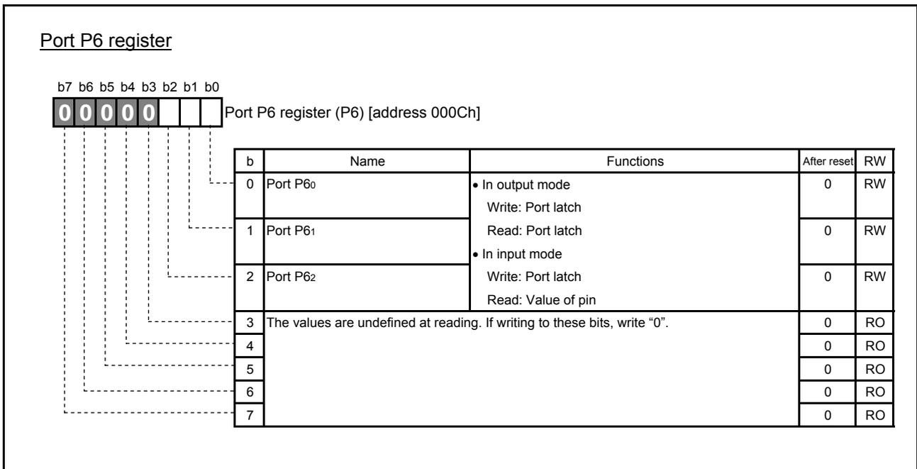
Fig. 4.2 Structure of Port P6 register
