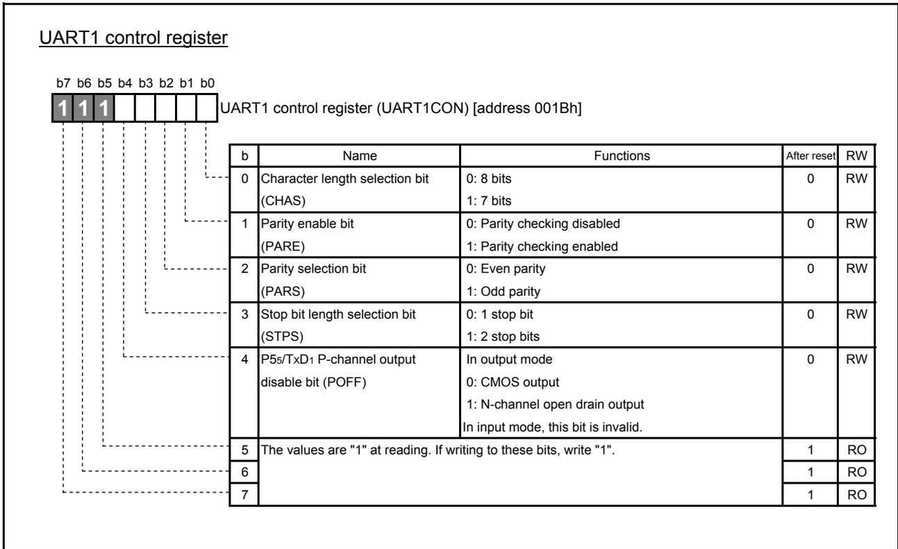
Fig. 4.16 Structure of UART1 control register
