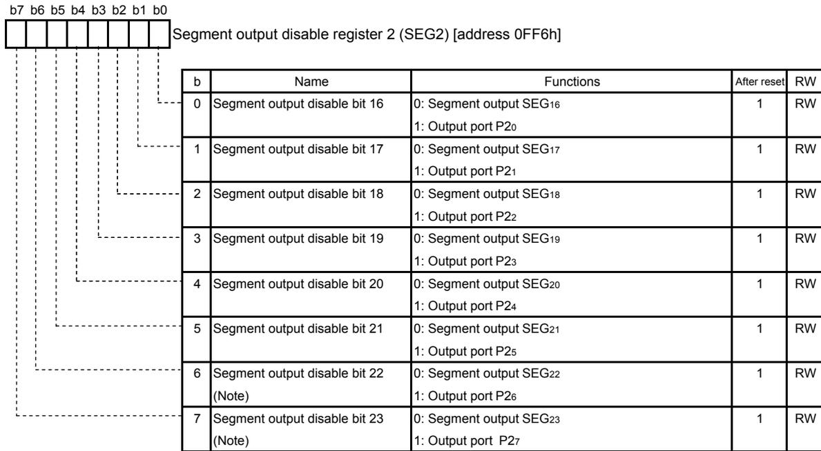
Note: When VL pin input selection bit (bit 5 at LCD power control register (address 0014h)) is set to "1", these bits become invalid.
