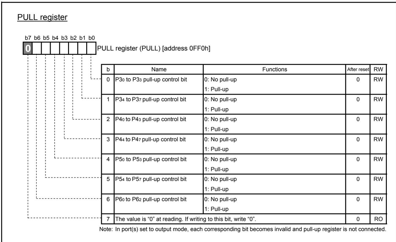
Fig. 4.47 Structure of PULL register
