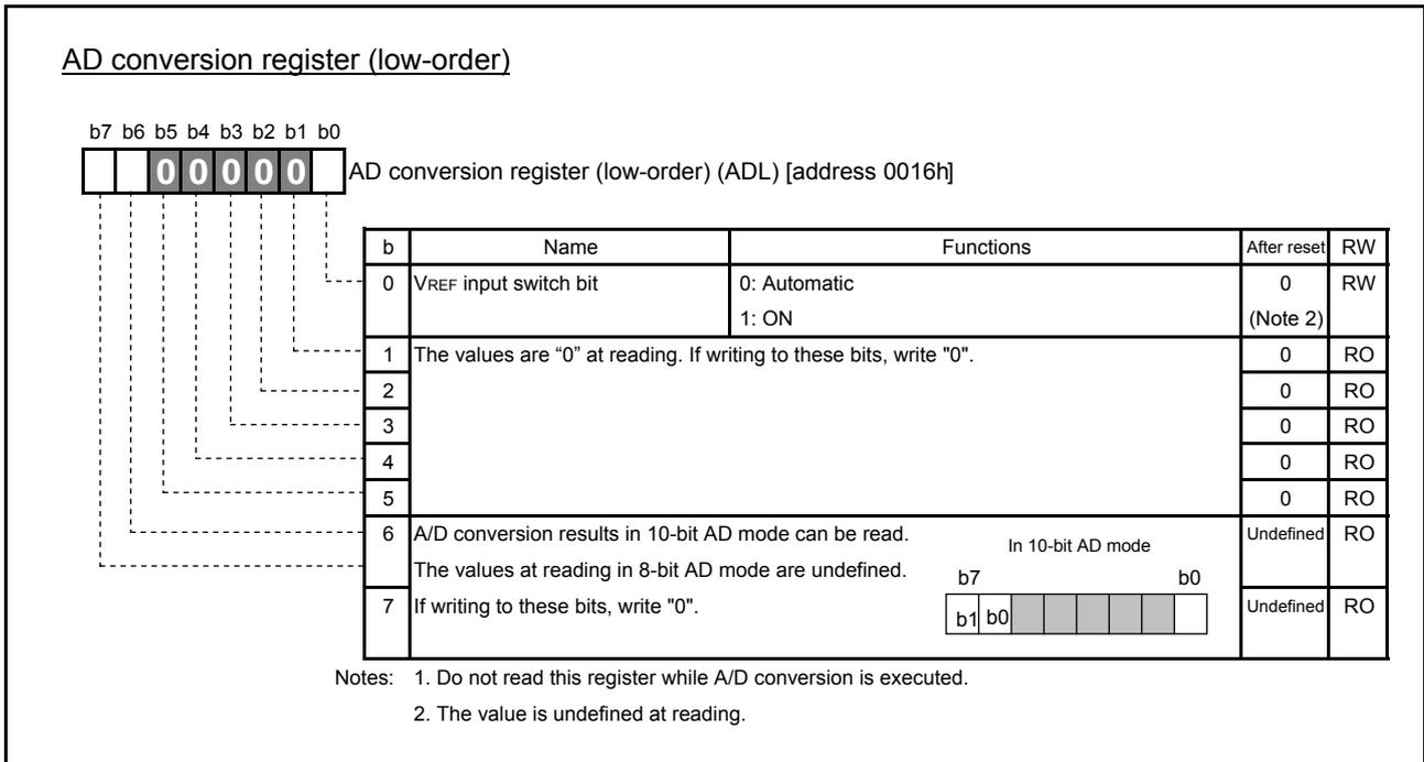
Fig. 4.11 Structure of AD conversion register (low-order)
