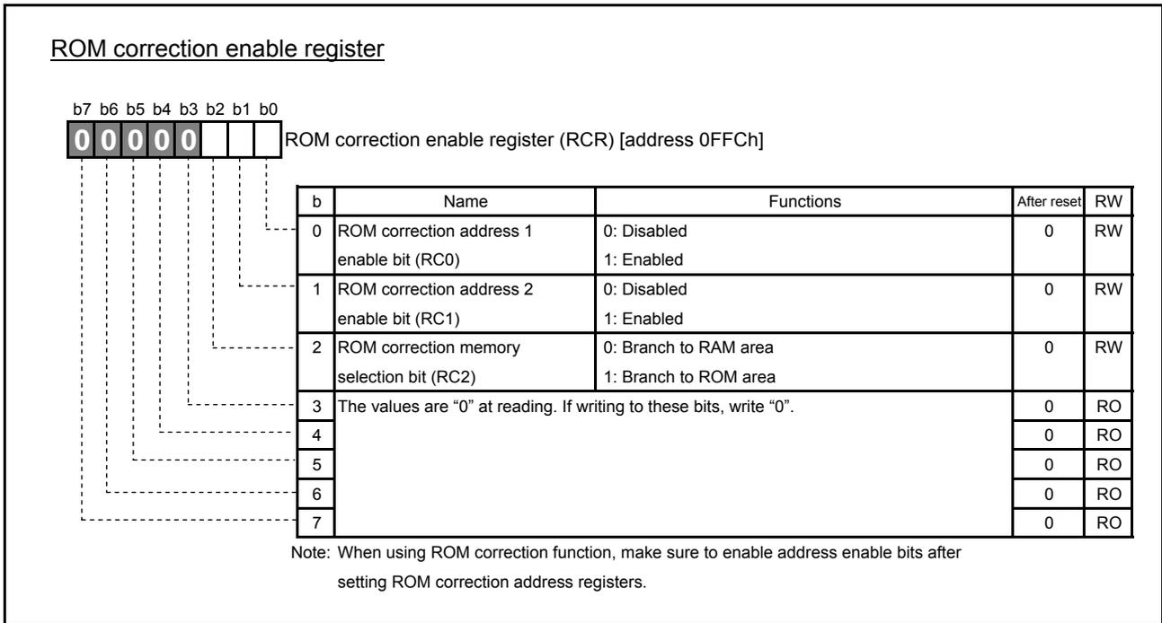
Fig. 4.58 Structure of ROM correction enable register
