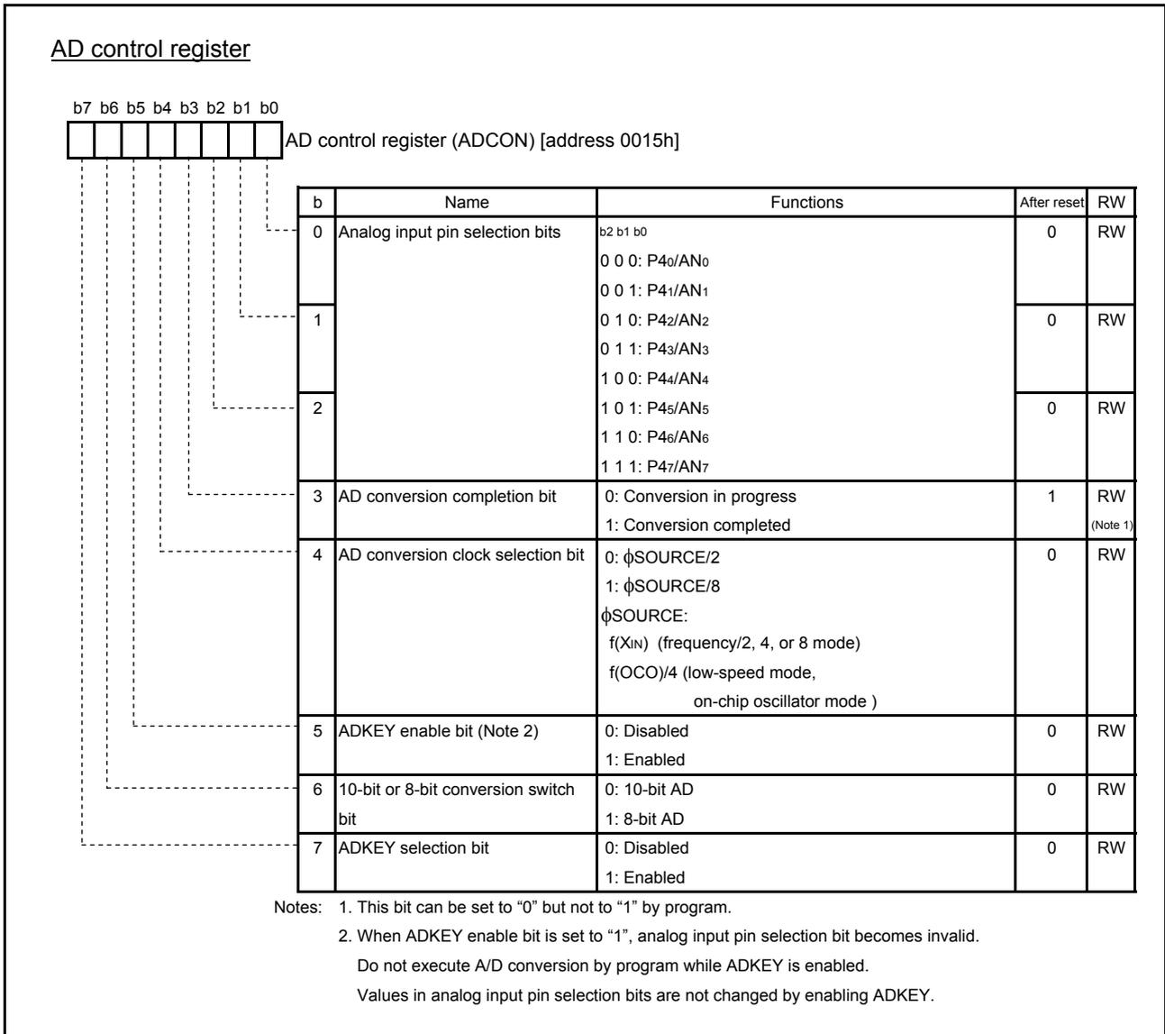
Fig. 4.10 Structure of AD control register
