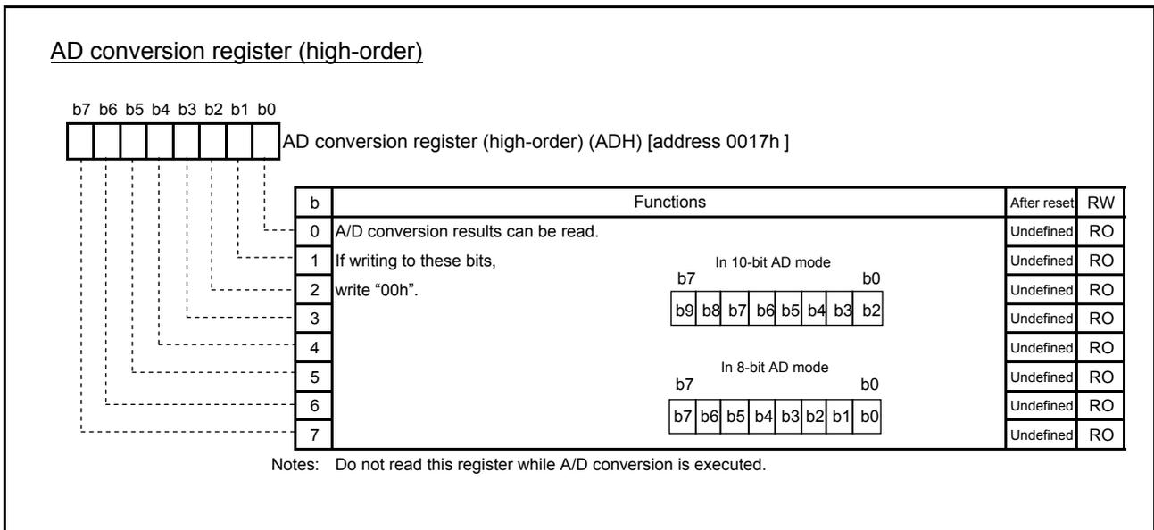
Fig. 4.12 Structure of AD conversion register (high-order)
