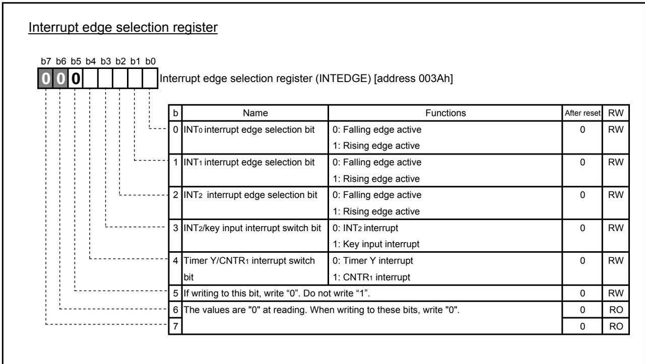
Fig. 4.40 Structure of interrupt edge selection register
