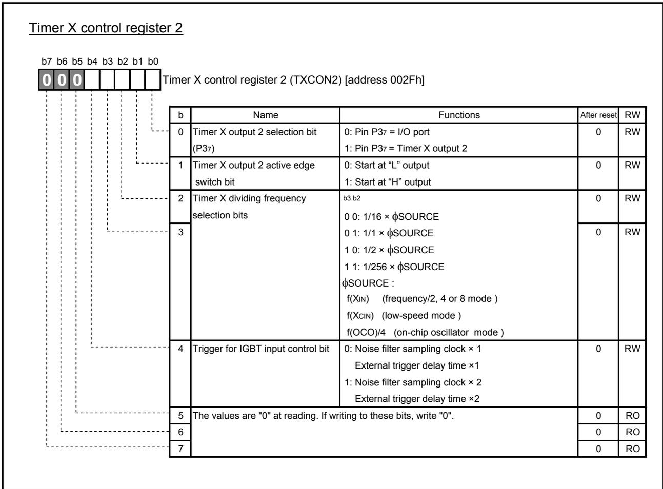
Fig. 4.35 Structure of Timer X control register 2
