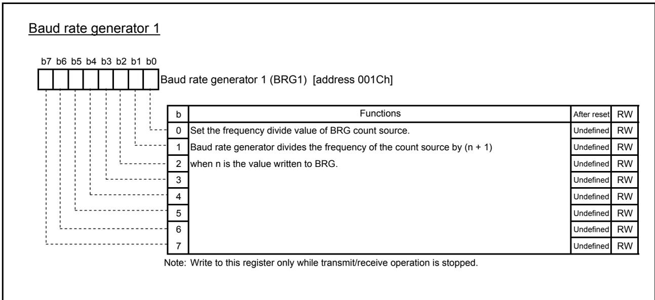
Fig. 4.17 Structure of Baud rate generator 1
