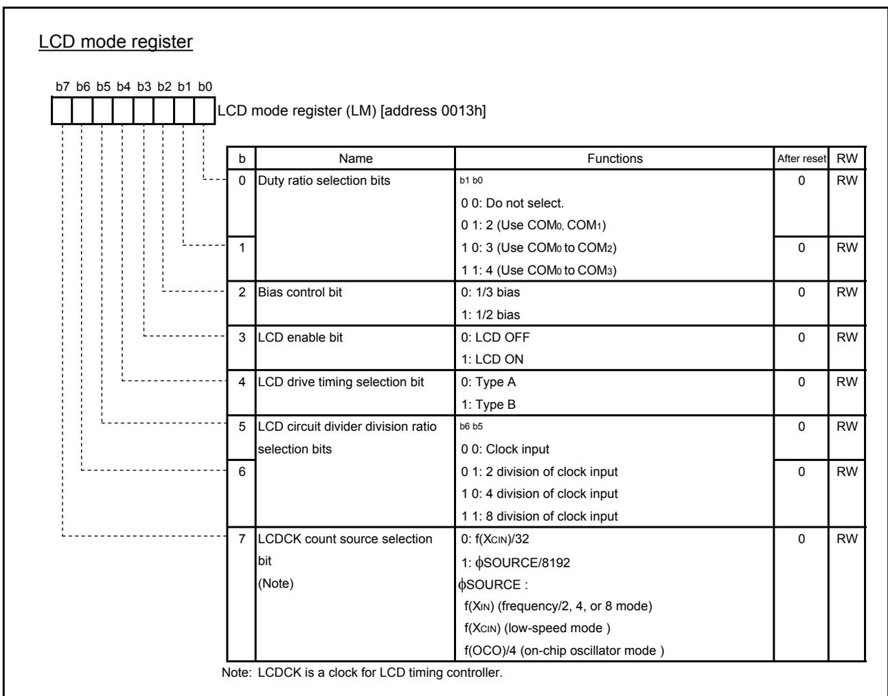
Fig. 4.8 Structure of LCD mode register
