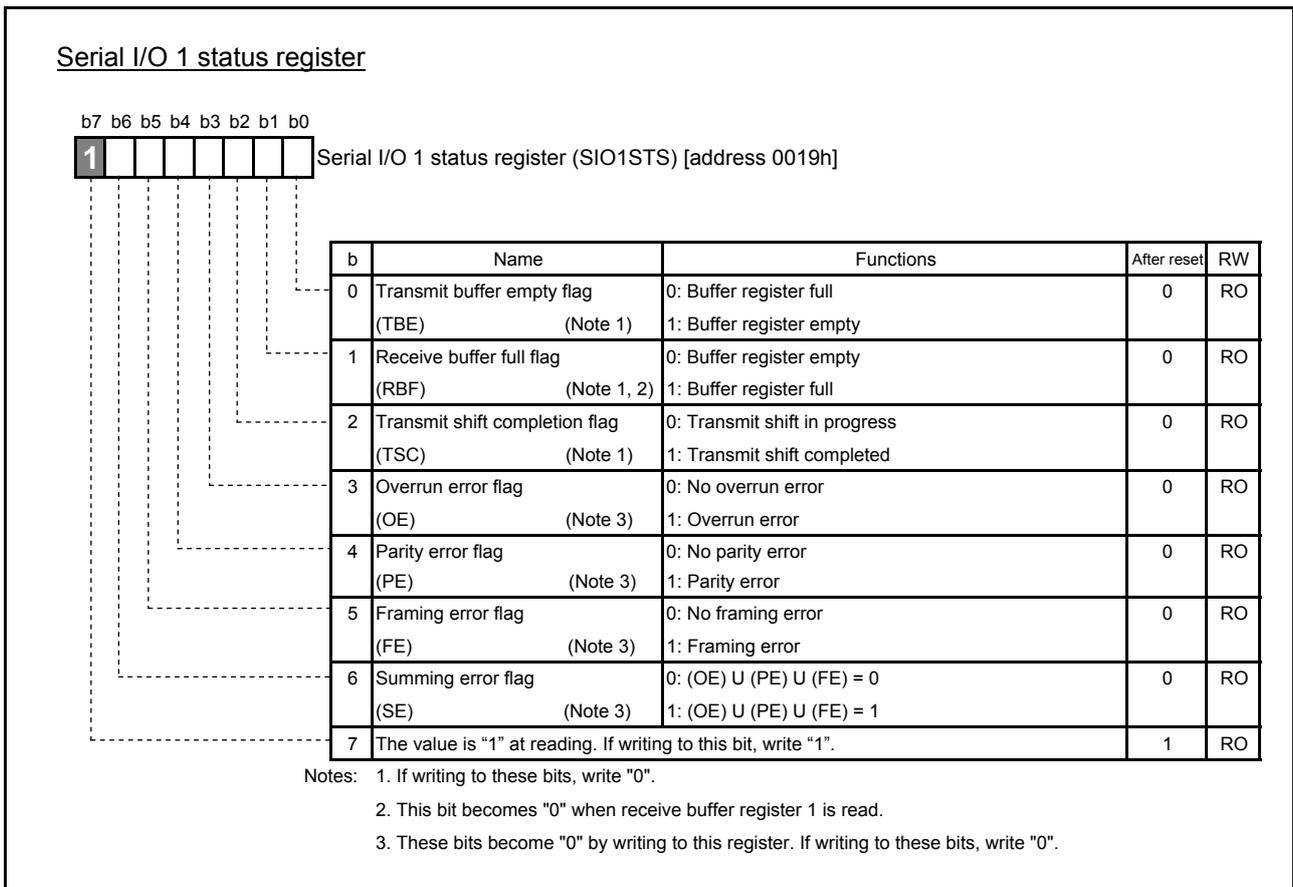
Fig. 4.14 Structure of serial I/O 1 status register
