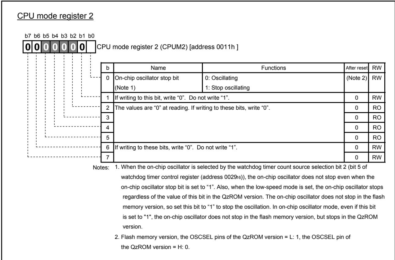
Fig. 4.6 Structure of CPU mode register 2
