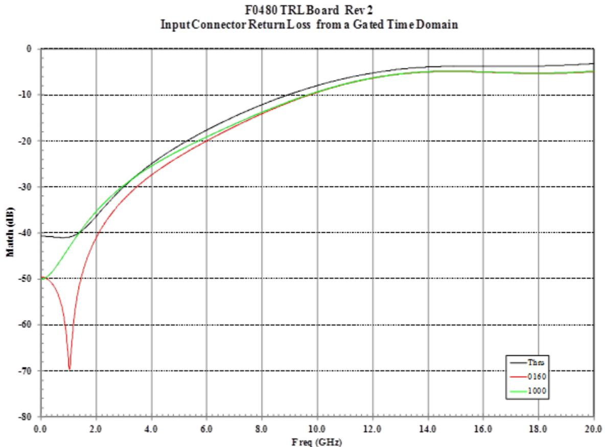
The input match is only for the connector and board connection. Using the gated response removed the resonance with the output connector. This shows that the inductance starts to become a factor around 2 GHz. Typically, the observance of a better than a -20 dB match would be desired if the measurements were being done at the connector.
