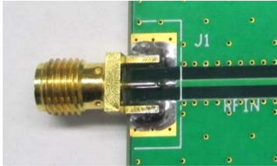
The advantage of performing time domain analysis is that response can be gated so that the response of only the particular time window selected is examined. This is done by setting the magnitude to zero, no discontinuity. Since we want to examine what the input connector and board connection is doing, we can gate the time domain response window from -0.2 to 0.2 ns. All other time is forced to zero. Because this is the first component in the circuit, masking concerns are not needed.
