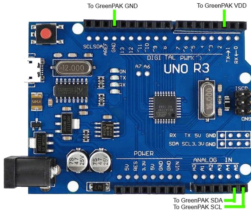
**Figure 1. Arduino Connections**
