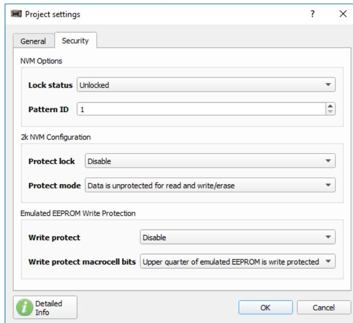
**Figure 9. Matrix Registers, NVM, and EEPROM Protection Settings**
