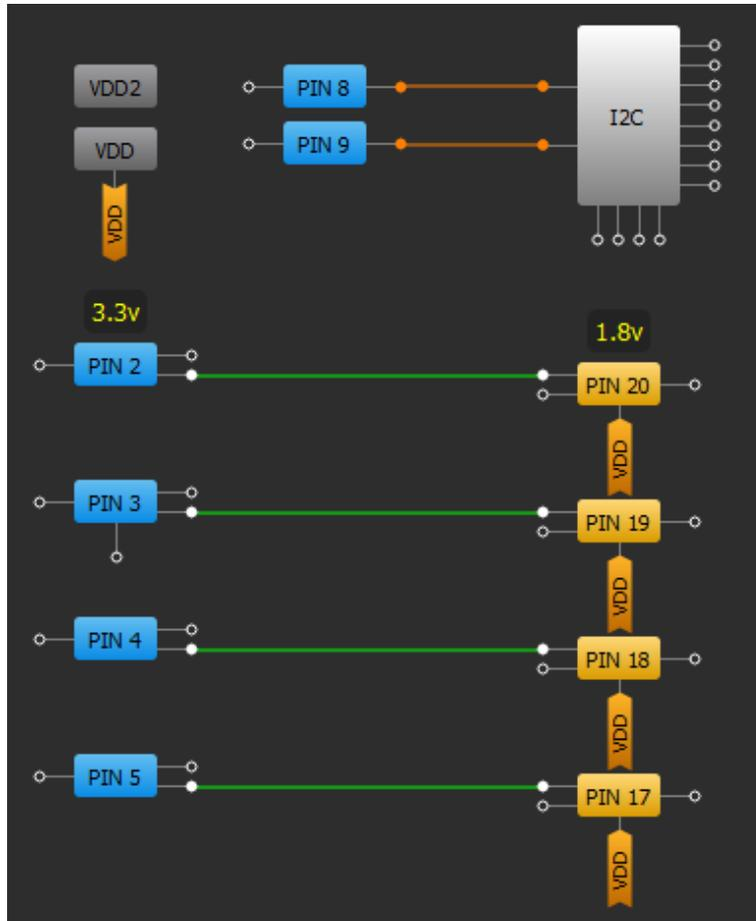
**Figure 2. Simple GreenPAK Design in a SLG46826**
