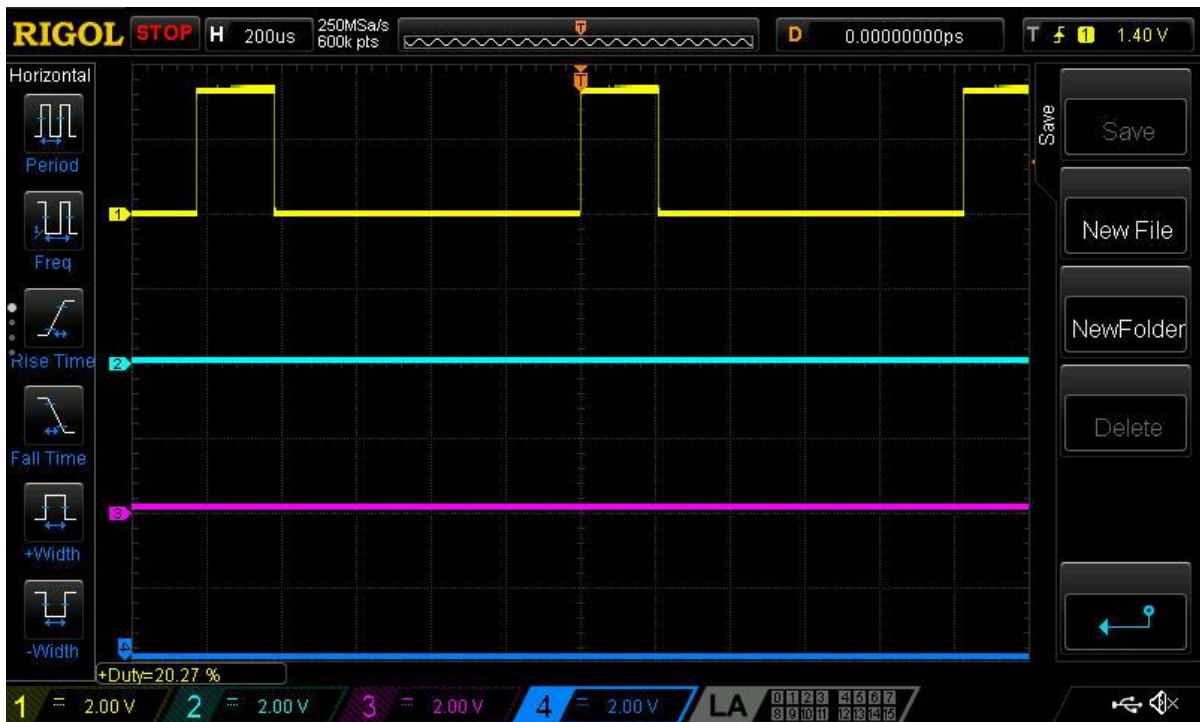
Figure 14: Minimum Limit of PWM Duty Cycle
