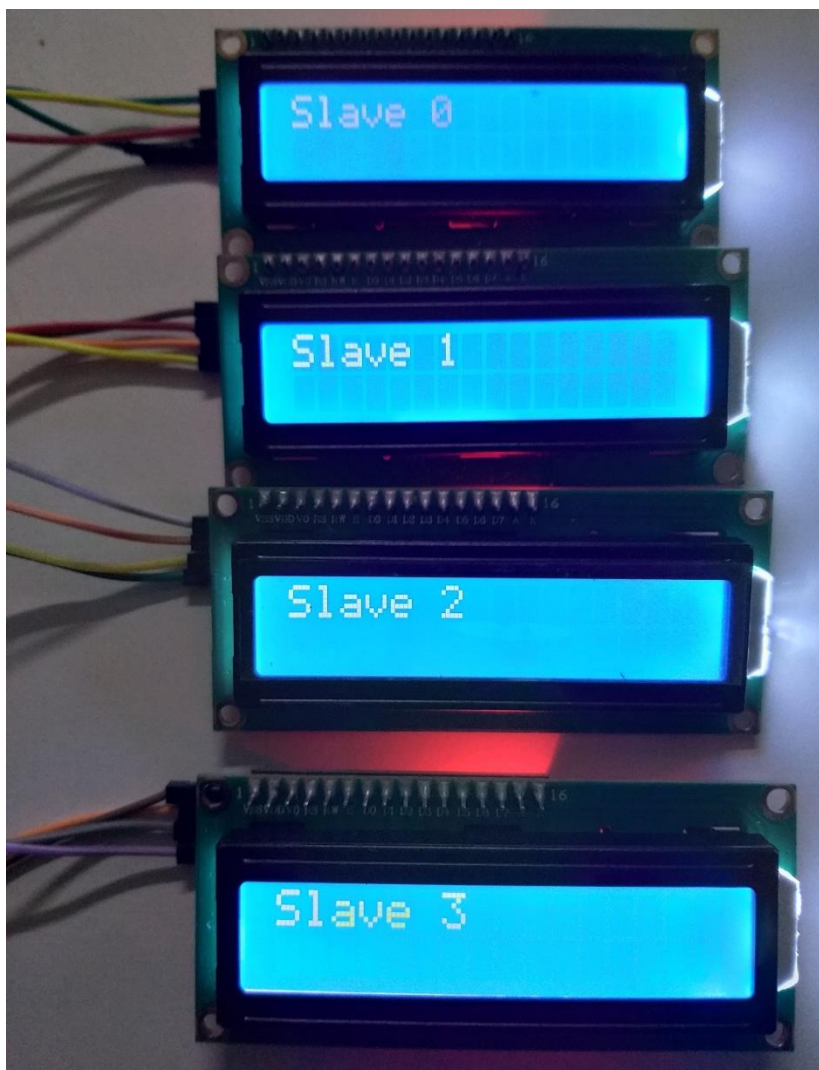
Figure 7: I 2 C-LCDs Outputs After Implementation
