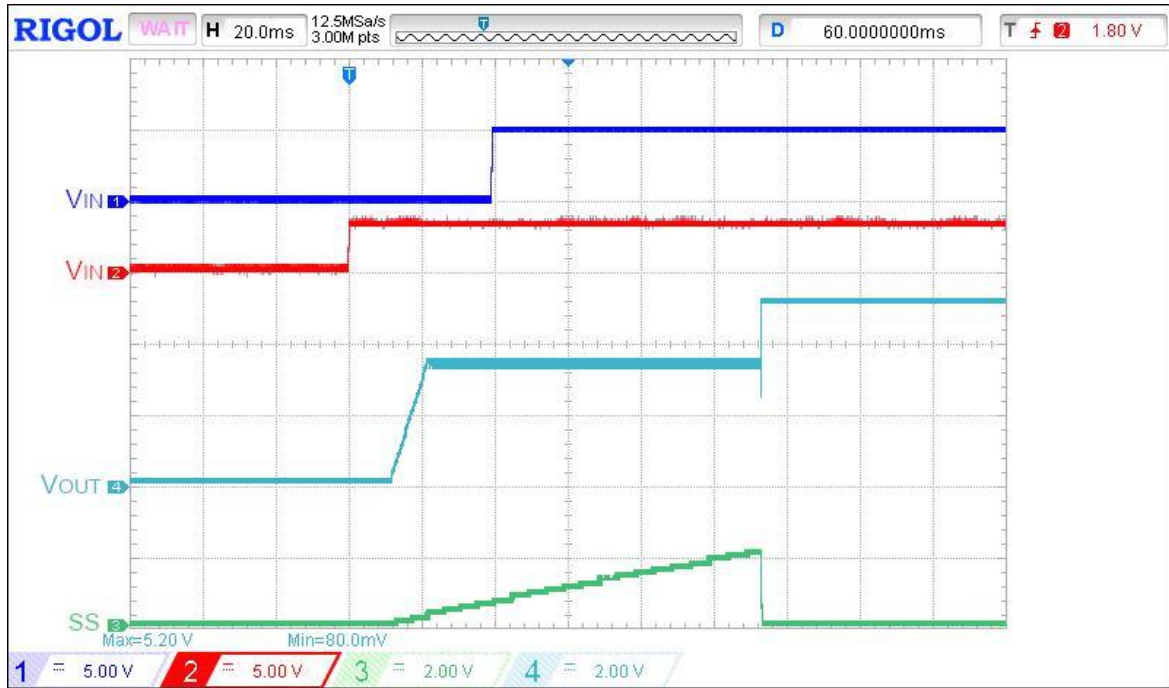
Figure 30: Higher voltage level priority operation waveform when V_{IN1} is applied before first SS rise is done for V_{IN1} = 5\text{ V} , V_{IN2} = 3.3\text{ V} , SEL = Low, PR = Low, C_{SS} = 220\text{ nF} , R_{LOAD} = 100\ \Omega , C_{LOAD} = 2\ \mu\text{F}
