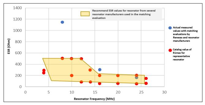
Figure 6. Group 3 and Group 5, Main clock: Resonator Frequency vs ESR max
