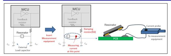
Figure 16. Measurement method of the oscillations excitation power
