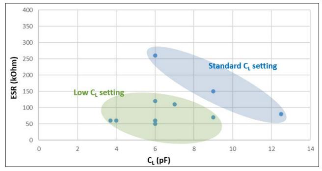
Figure 12. Group 6, Sub-clock: C<sub>L</sub> vs ESR max
