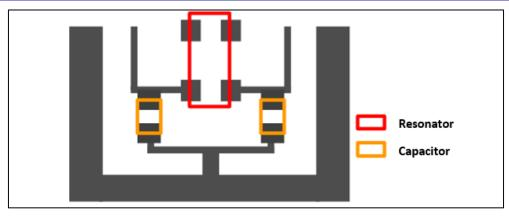
Figure 22. Pattern example when two external capacitors are difficult to place near MCU
