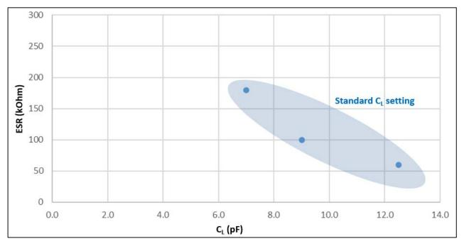
Figure 5. Group 2, Sub-clock: C<sub>L</sub> vs ESR max
