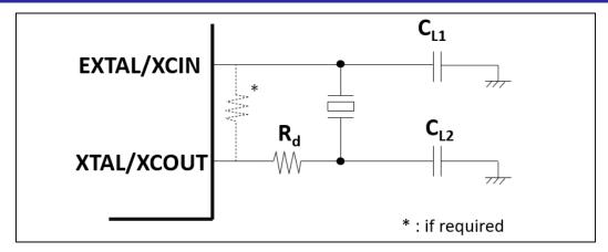
Figure 1. Connection Example of External Resonator
