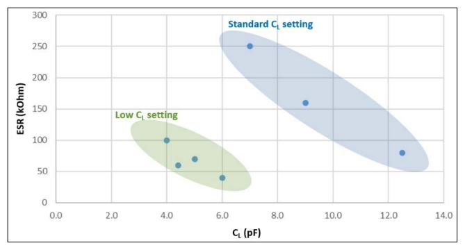
Figure 3. Group 1, Sub-clock: C<sub>L</sub> vs ESR max
