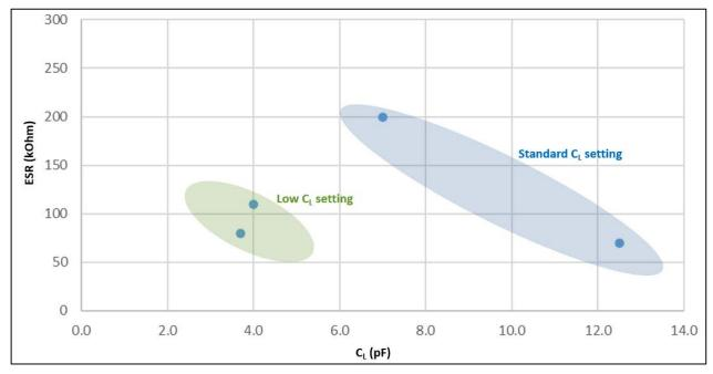
Figure 7. Group 3, Sub-clock: C<sub>L</sub> vs ESR max
