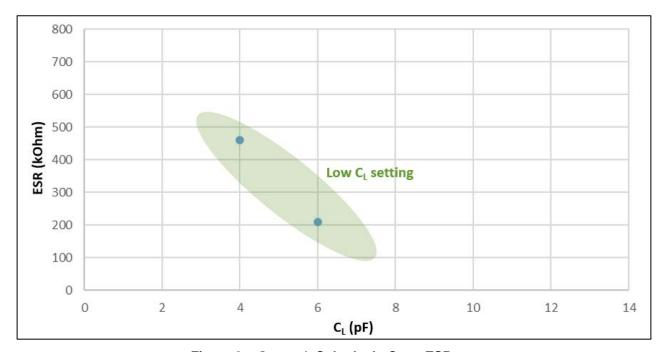
Figure 9. Group 4, Sub-clock: C<sub>L</sub> vs ESR max
