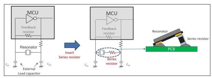
Figure 15. Measurement method of the negative resistance
