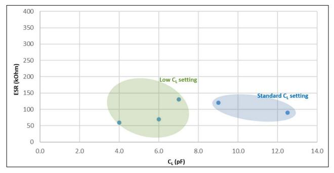
Figure 14. Group 7, Sub-clock: C<sub>L</sub> vs ESR max
