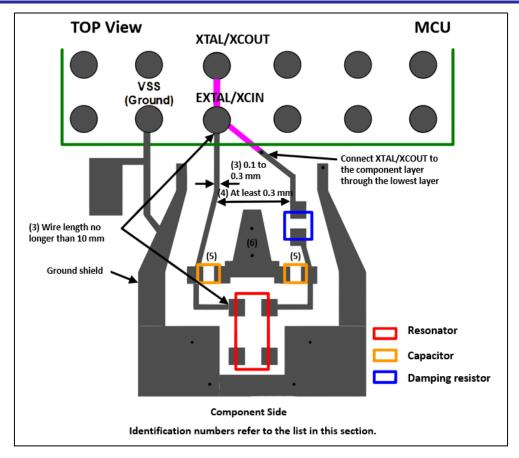
Figure 20. Example of the EXTAL/XCIN and XTAL/XCOUT Routing Pattern: LGA Package
