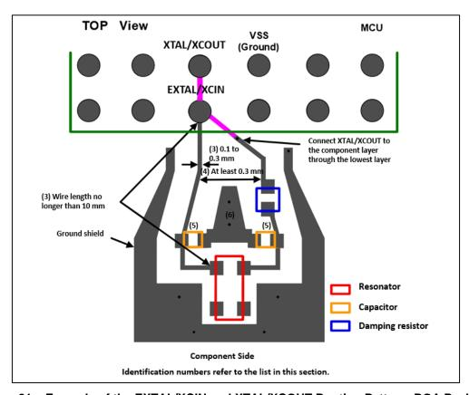
Figure 21. Example of the EXTAL/XCIN and XTAL/XCOUT Routing Pattern: BGA Package
