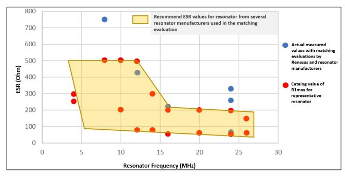
Figure 2. Group 1, Main clock: Resonator Frequency vs ESR max
