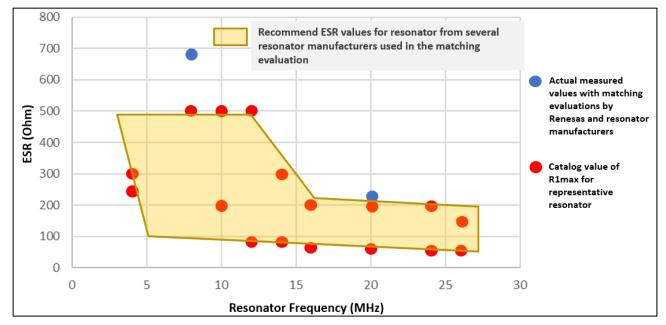
Figure 11. Group 6, Main clock: Resonator Frequency vs ESR max
