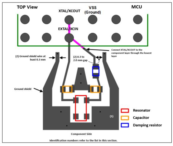
Figure 25. Example of the ground shield tracing: BGA Package
