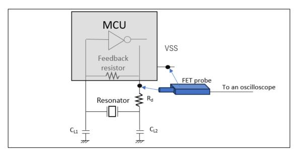
Figure 17. Oscillation Amplitude Voltage Measurement Method
