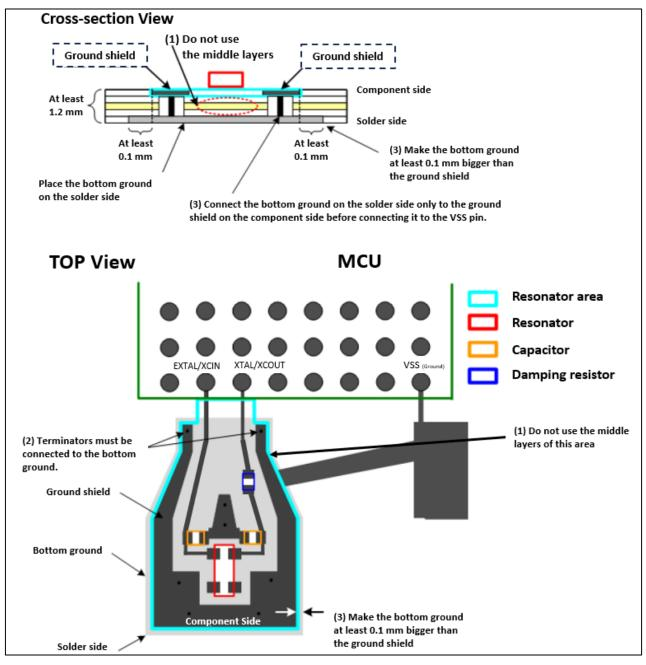
Figure 28. Routing example for a multilayered board thicker than 1.2 mm: LGA/BGA Package (VSS is placed in the outer column)
