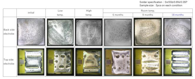
Figure 4 Representative electrode photo after soldering
