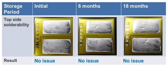
Figure 6 Representative electrode photo after soldering
