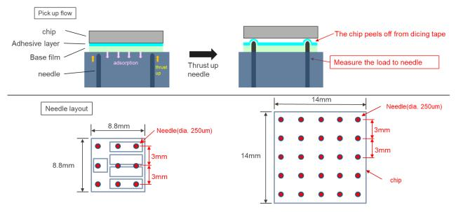
Figure 2 Measuring method for Pickup intensity
