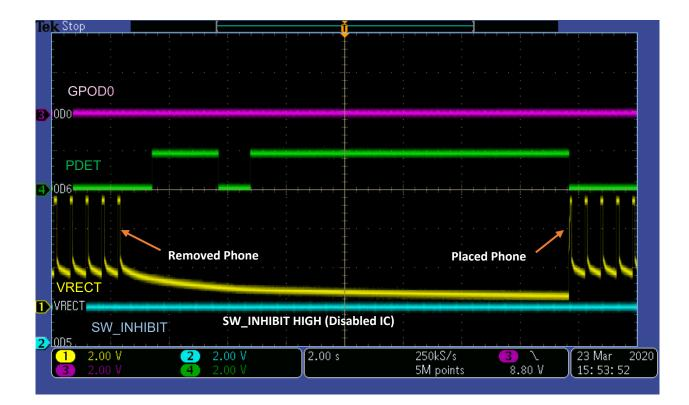
Figure 3. Waveform of PDET (OD6) Output Indicating Rx Removal and Placement with SW\_Inhibited.
