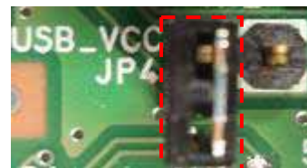
Power supply “OFF” (Open) setting
