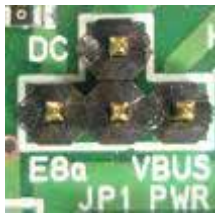
Figure 3 JP1 Main power supply switch
