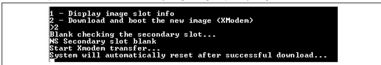
**Figure 78. Choose Option 2 to Download the New Image using XModem**
