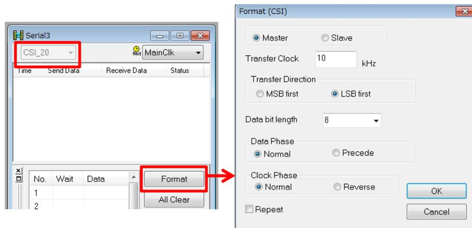
Figure 33 Serial Window (CSI20) 1/2
