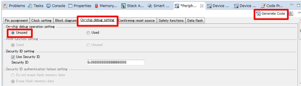
Figure 10 On-Chip Debug Operation Setting
