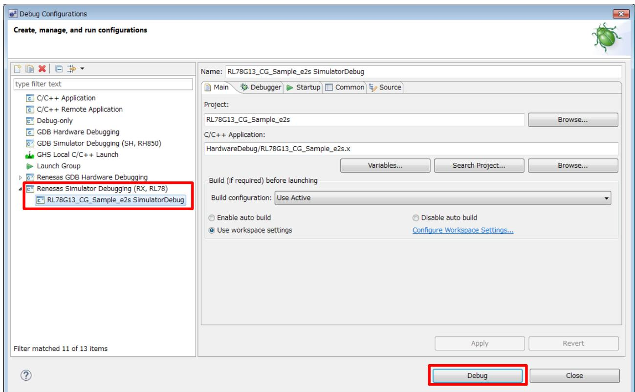
Figure 13 Debug Configuration
