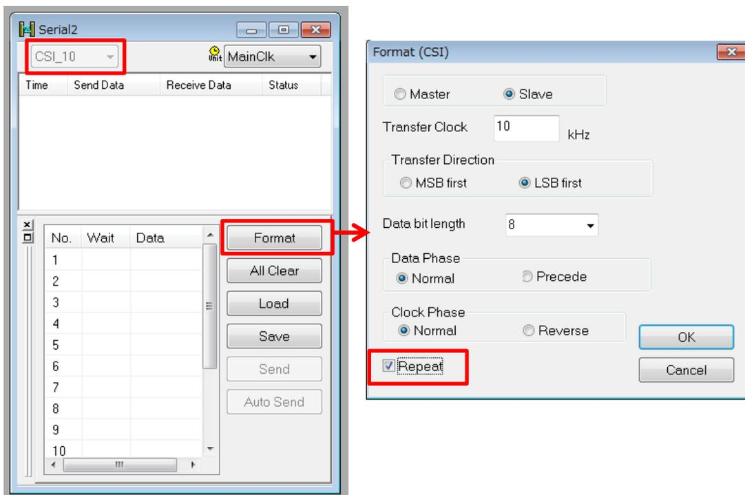
**Figure 31 Serial Window (CSI10) 1/2**
