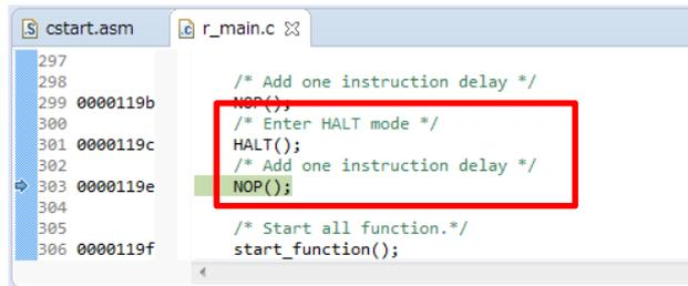
Figure 40 Where the program halted (when transitioning to HALT mode)
