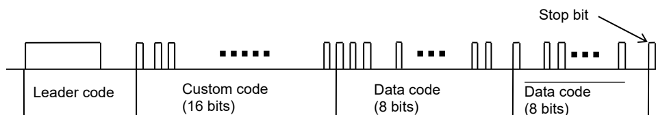
Figure5-1 Example of NEC Format for Infrared Remote Control
