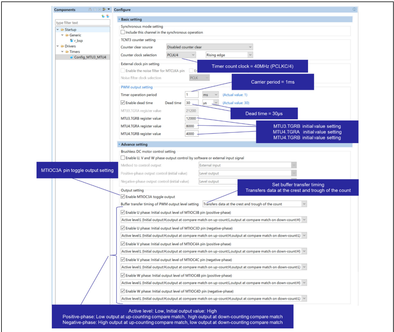
Figure 3.55 MTU3 and MTU4 Settings (1/2)
