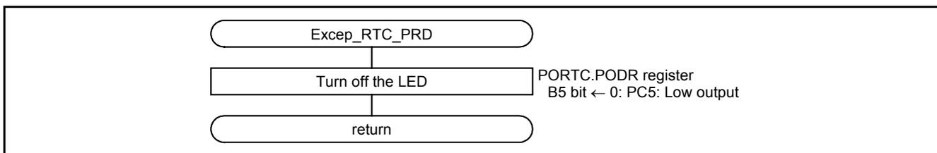
Figure 5.12 RTC Period Interrupt Handling
