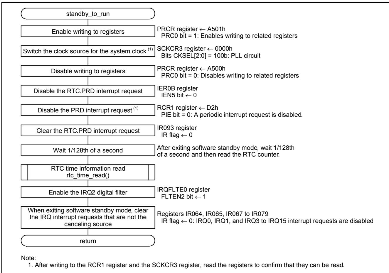
Figure 5.11 Exiting Software Standby Mode
