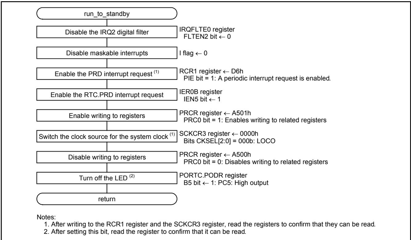
Figure 5.10 Preparation to Enter Software Standby Mode
