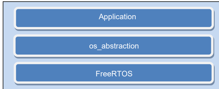
Figure 3-1 OS Hierarchical Software Layers
