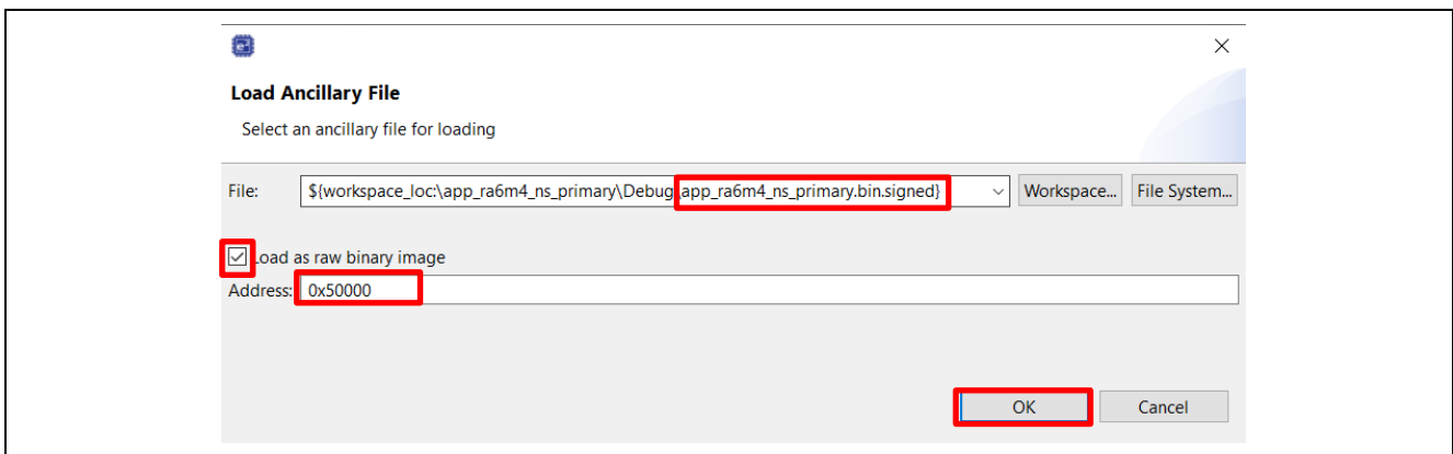
Figure 22. Load the Primary Non-Secure Image to the Second Slot
