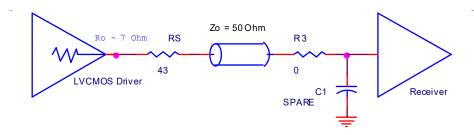
Figure 4. One-to-One LVCMOS Series Termination
