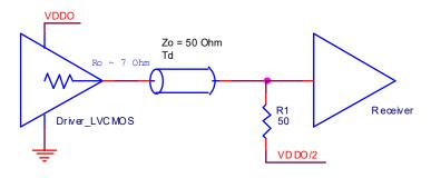
Figure 1. LVCMOS Driver Standard Termination
