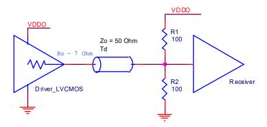
Figure 2. LVCMOS Parallel Termination
