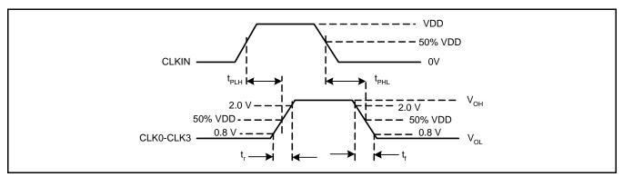
Figure 2. Voltage Thresholds for Propagation Delay  $(t_{pd})$  Measurements
