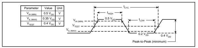
Figure 4. Clock Waveform
