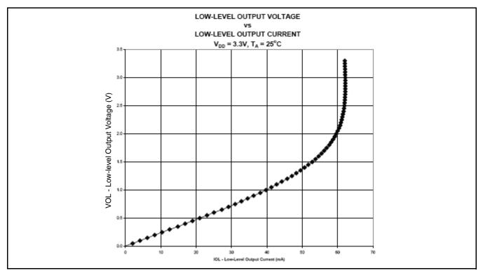
Figure 7. Low-level Output Voltage vs. Low-level Output Current
