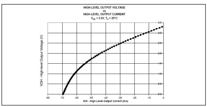
Figure 6. High-level Output Voltage vs. High-level Output Current
