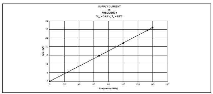
Figure 5. Supply Current vs. Frequency
