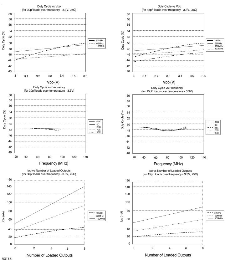
1. Duty Cycle is taken from typical chip measured at 1.4V.
