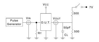
Test Circuits for All Outputs
