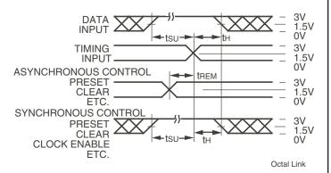
Set-Up, Hold, and Release Times
