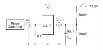
Test Circuits for All Outputs
