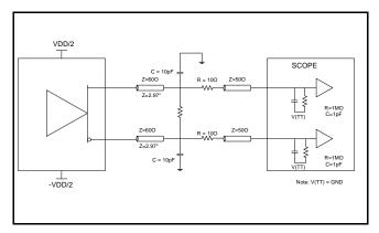
Figure 2: Output load test circuit
