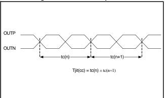
Figure 3: Cycle-cycle jitter
