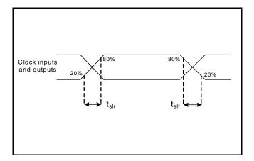
Figure 5: Input and Output Slew Rates
