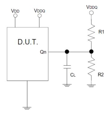
Test Circuit for SDR Outputs
