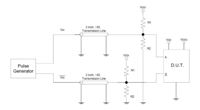
Test Circuit for Differential Input<sup>(1)</sup>
