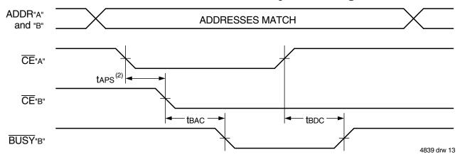
Waveform of  $\overline{\textbf{BUSY}}$  Arbitration Cycle Controlled by Address Match Timing (M/ $\overline{\textbf{S}}$  = VIH)<sup>(1)</sup>
