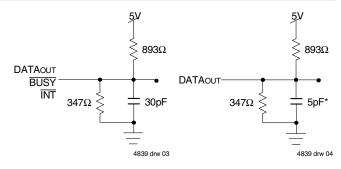
Figure 1. AC Output Test Load
