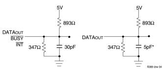
Figure 1. AC Output Test Load
