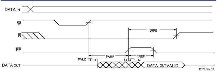
Figure 17. Read Data Flow-Through Mode
