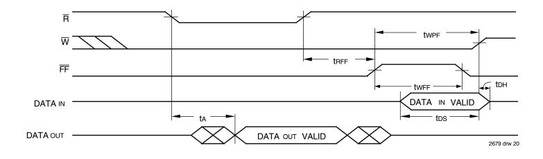
Figure 18. Write Data Flow-Through Mode
