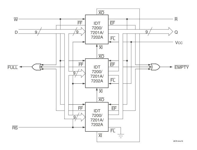
Figure 14. Block Diagram of 768 x 9, 1,536 x 9, 3,072 x 9 FIFO Memory (Depth Expansion)
