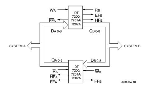
Figure 16. Bidirectional FIFO Mode
