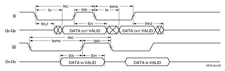
Figure 3. Asynchronous Write and Read Operation
