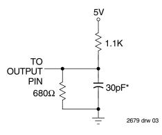
or equivalent circuit *Figure 1. Output Load* \* Includes scope and jig capacitances.
