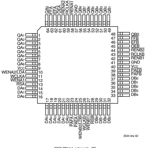
TQFP (PN64-1, order code: PF) STQFP (PP64-1, order code: TF) TOP VIEW
