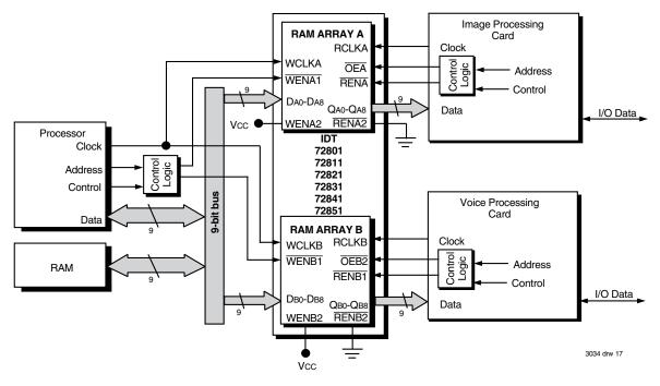
Figure 16. Block Diagram of Two Priority Configuration
