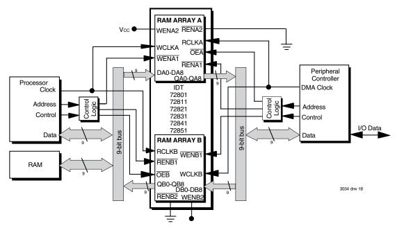
Figure 17. Block Diagram of Bidirectional Configuration
