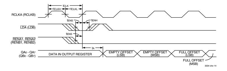
Figure 13. Read Offset Register Timing
