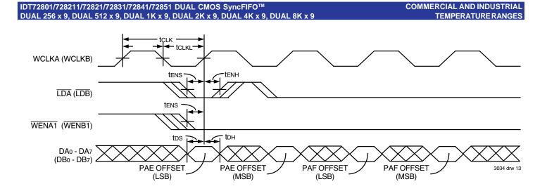
Figure 12. Write Offset Register Timing
