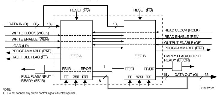
Figure 29. Block Diagram of the two FIFOs contained in one IDT72805LB/72815LB/72825LB/72845LB configured for a 36-bit Width Expansion
