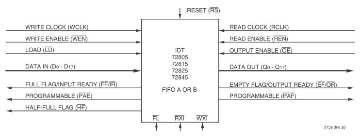
Figure 28. Block Diagram of Single 256 x 18, 512 x 18, 1,024 x 18, 4,096 x 18 Synchronous FIFO (One of the two FIFOs contained in the IDT72805LB/72815LB/72825LB/72845LB)
