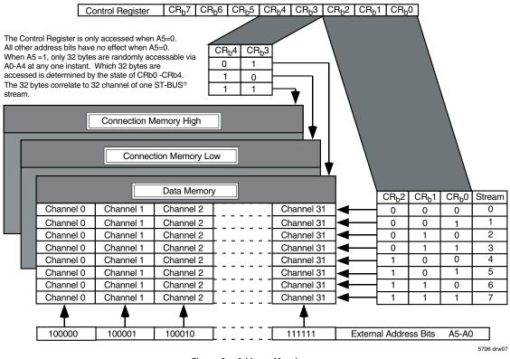
Figure 3. Address Mapping
