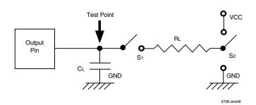
S1 is open circuit except when testing output levels or high impedance states.
