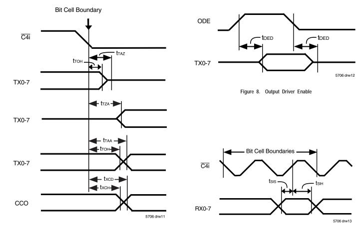
Figure 7. Serial Outputs and External Control
