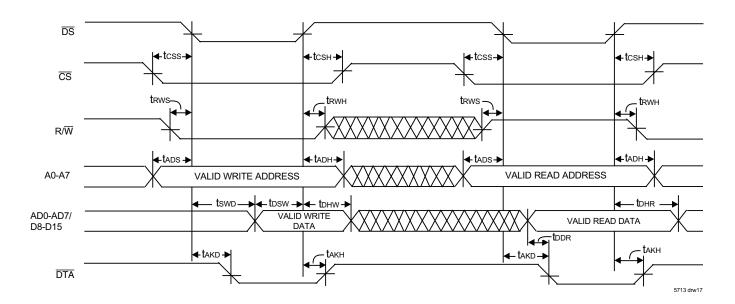
Figure 14. Motorola Non-Multiplexed Asyncronous Bus Timing
