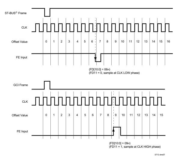
Figure 4. Example for Frame Alignment Measurement
