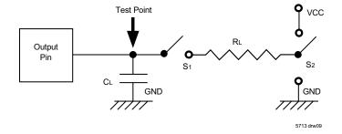
Figure 6. Output Load
