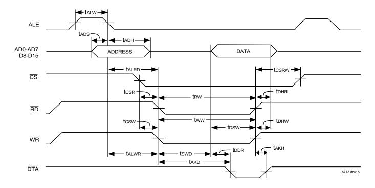
Figure 12. Multiplexed Bus Timing (Intel Mode)
