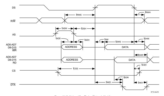
Figure 13. Multiplexed Bus Timing (Motorola Mode)
