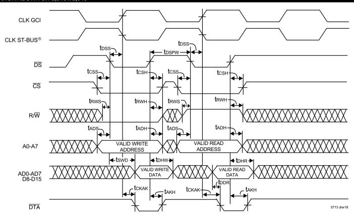
Figure 15. Motorola Non-Multiplexed Syncronous Bus Timing
