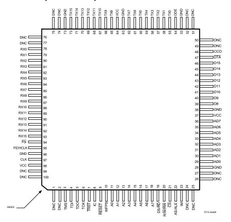
TQFP: 0.50mm pitch, 14mm x 14mm (PN100-1, order code: PF)
