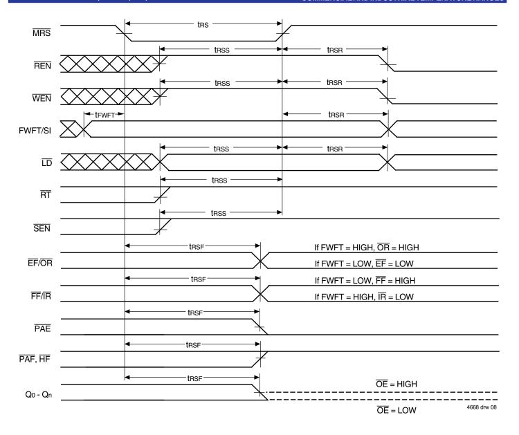
Figure 5. Master Reset Timing
