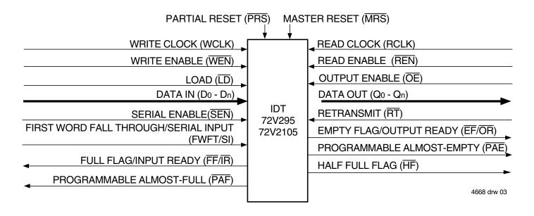
Figure 1. Block Diagram of Single 131,072 x 18 and 262,144 x 18 Synchronous FIFO
