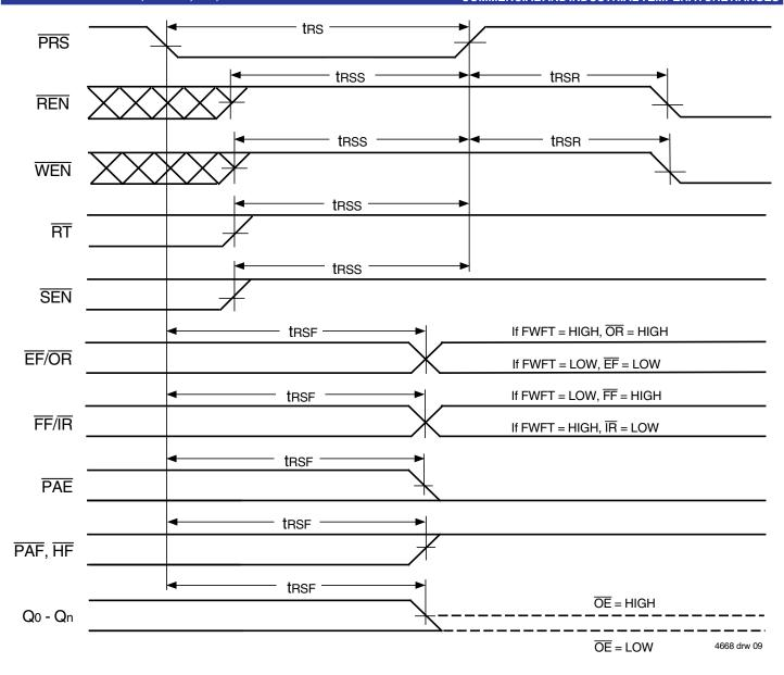
Figure 6. Partial Reset Timing
