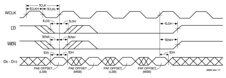
Figure 14. Parallel Loading of Programmable Flag Registers (IDT Standard and FWFT Modes)
