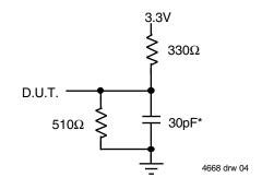
Figure 2. Output Load
