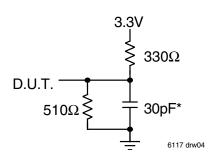
Figure 2a. Output Load
