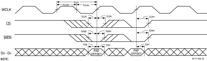
1. This timing diagram illustrates programming with an input bus width of 36 bits.
