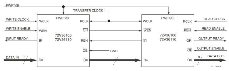
Figure 30. Block Diagram of 131,072 x 36 and 262,144 x 36 Depth Expansion
