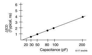
Figure 2c. Lumped Capacitive Load, Typical Derating
