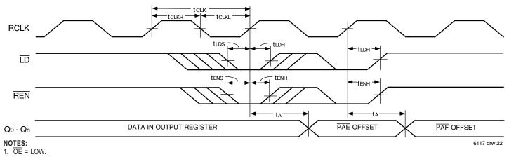
2. The timing diagram illustrates reading of offset registers with an output bus width of 36 bits.
