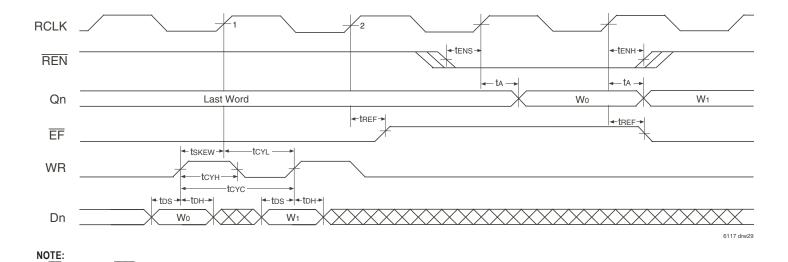
Figure 24. Asynchronous Write, Synchronous Read, Empty Flag Operation (Standard Mode)
