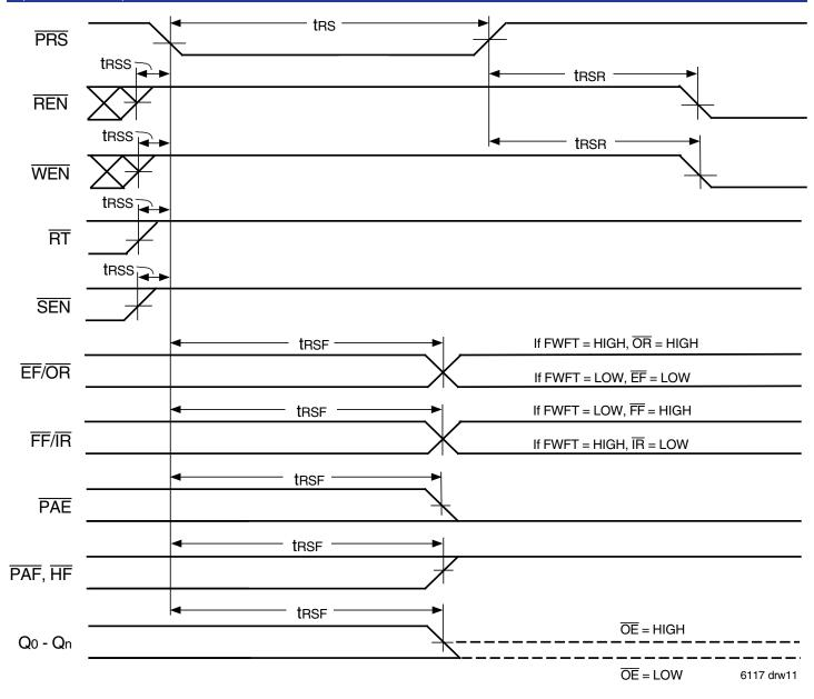
Figure 6. Partial Reset Timing
