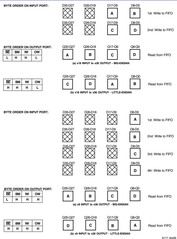
Figure 4. Bus-Matching Byte Arrangement (Continued)
