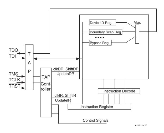
Figure 32. Boundary Scan Architecture
