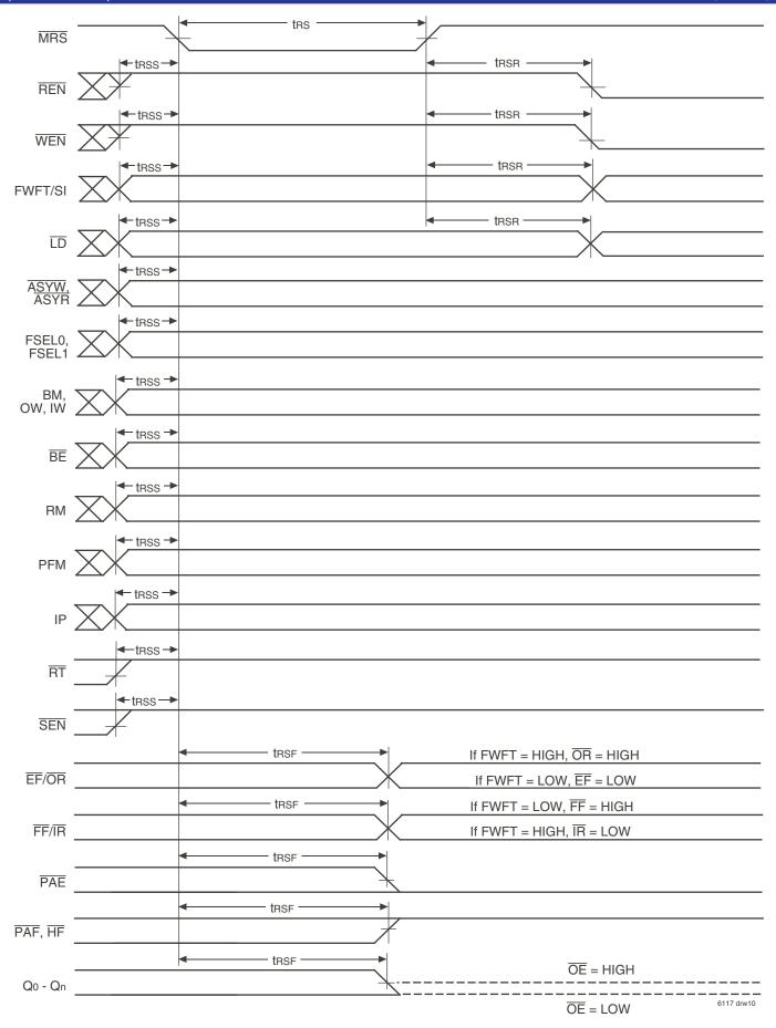
Figure 5. Master Reset Timing
