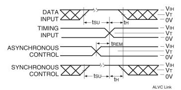
Set-up, Hold, and Release Times
