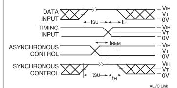
Set-up, Hold, and Release Times
