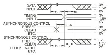
Set-up, Hold, and Release Times
