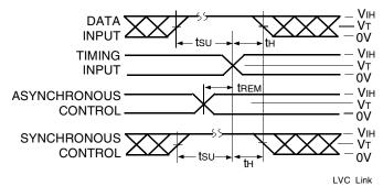
Set-up, Hold, and Release Times
