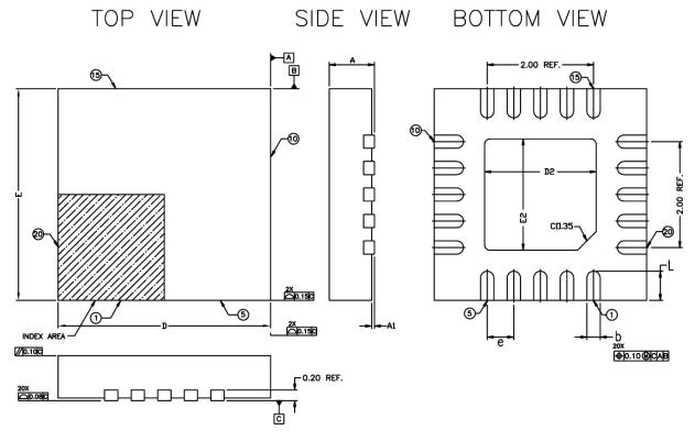
Table 8. Package Dimensions for 20-Lead VFQFN
