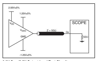
3.3V Core/2.5V Output Load Test Circuit
