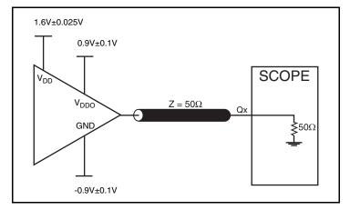
2.5V Core/1.8V Output Load Test Circuit
