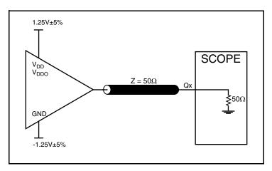
2.5V Core/2.5V Output Load Test Circuit
