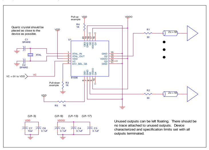
Figure 2. 81006 Schematic Example
