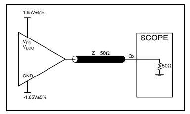
3.3V Core/3.3V Output Load Test Circuit
