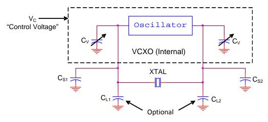
Figure 1. VCXO Oscillator Circuit
