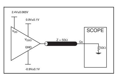
3.3V Core/1.8V Output Load Test Circuit
