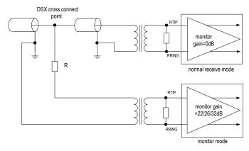
Figure-9 Monitoring Receive Line in Another Chip
