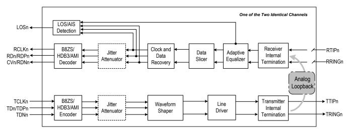
Figure-14 Analog Loopback
