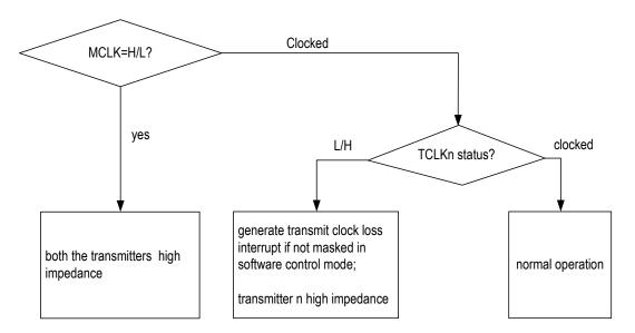
Figure-19 TCLK Operation Flowchart
