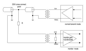
Figure-10 Monitor Transmit Line in Another Chip
