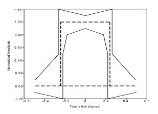
Figure-3 E1 Waveform Template Diagram
