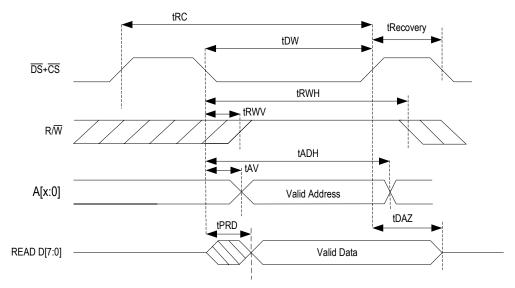
Figure-33 Non\_multiplexed Motorola Read Timing
