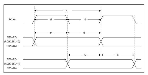
Figure-24 Receive System Interface Timing
