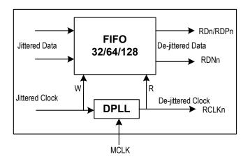
Figure-12 Jitter Attenuator
