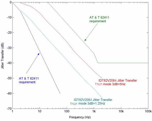
Figure-28 T1/J1 Jitter Transfer Performance
