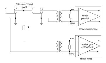
Figure-9 Monitoring Receive Line in Another Chip
