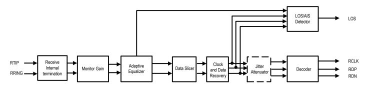
Figure-7 Receive Path Function Block Diagram
