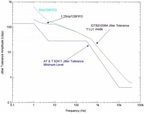
Figure-26 T1/J1 Jitter Tolerance Performance
