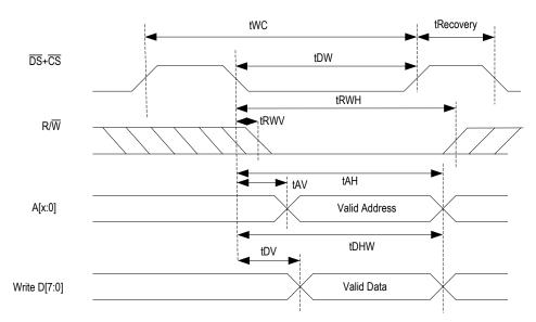
Figure-34 Non\_multiplexed Motorola Write Timing
