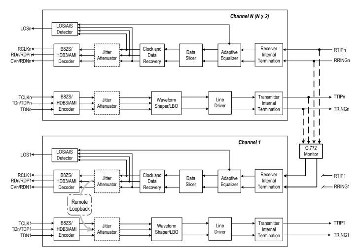
Figure-11 G.772 Monitoring Diagram
