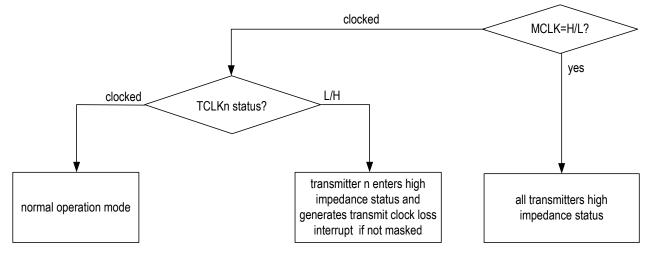
Figure-19 TCLK Operation Flowchart
