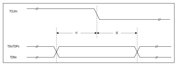
Figure-23 Transmit System Interface Timing
