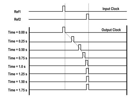
Figure - 6 Reference Switch with TIE Control Block Disabled
