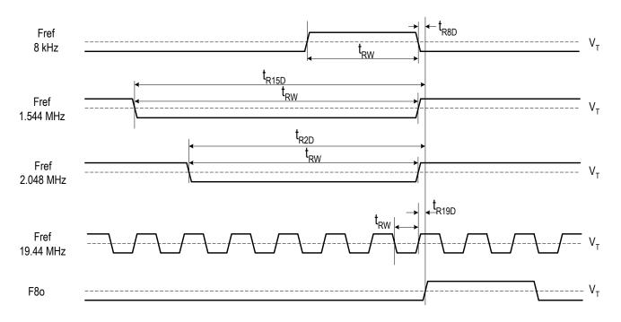
Figure - 12 Input to Output Timing (Normal Mode)
