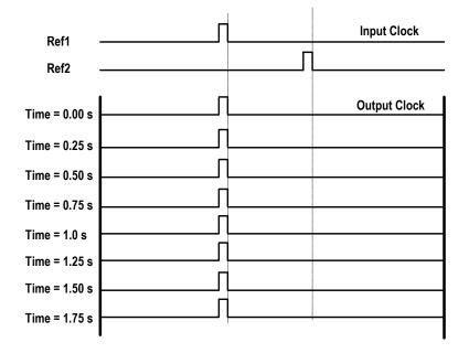
Figure - 5 Reference Switch with TIE Control Block Enabled
