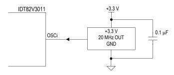
Figure - 8 Clock Oscillator Circuit
