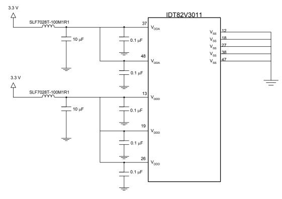
Figure - 10 IDT82V3011 Power Decoupling Scheme
