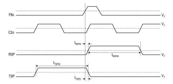
Figure - 14 Output Timing 2
