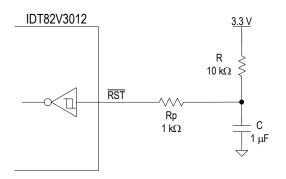
Figure - 9 Power-Up Reset Circuit
