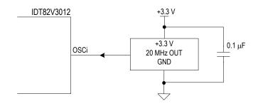
Figure - 8 Clock Oscillator Circuit
