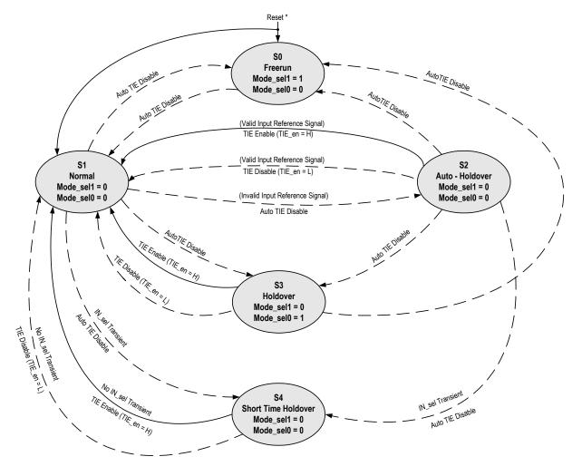
$<sup>^{\</sup>star}$  Note: After reset, the Mode\_sel1 and Mode\_sel0 should be initially set to '10' or '00'.
