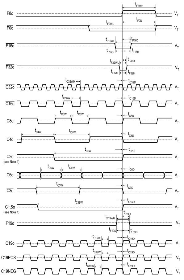
Figure - 13 Output Timing 1
