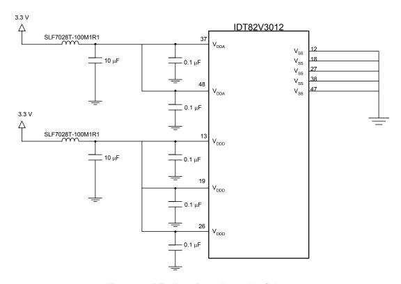
Figure - 10 IDT82V3012 Power Decoupling Scheme
