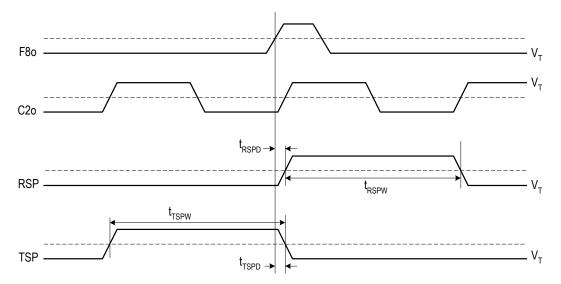
Figure - 14 Output Timing 2
