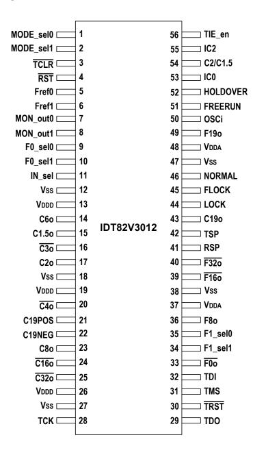
Figure - 1 IDT82V3012 SSOP56 Package Pin Assignment
