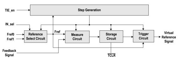
Figure - 4 TIE Control Block Diagram
