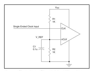
Figure 1. Single-Ended Signal Driving Differential Input
