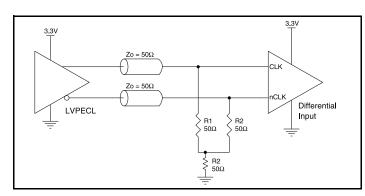
Figure 2B. HiPerClockS CLK/nCLK Input Driven by a 3.3V LVPECL Driver
