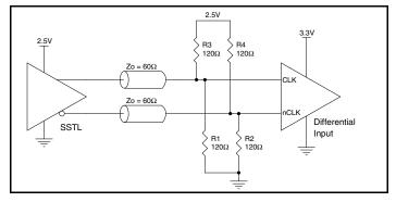
Figure 2F. HiPerClockS CLK/nCLK Input Driven by a 2.5V SSTL Driver
