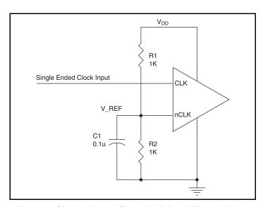
Figure 1. Single-Ended Signal Driving Differential Input
