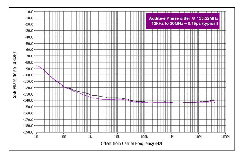
As with most timing specifications, phase noise measurements has issues relating to the limitations of the equipment. Often the noise floor of the equipment is higher than the noise floor of the device. This is illustrated above. The device meets the noise floor
