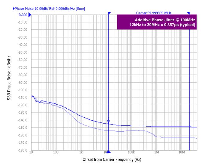
As with most timing specifications, phase noise measurements has issues relating to the limitations of the equipment. Often the noise floor of the equipment is higher than the noise floor of the device. This is illustrated above. The device meets the noise floor of what is shown, but can actually be lower.
