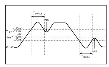
**Differential Measurement Points for Ringback**
