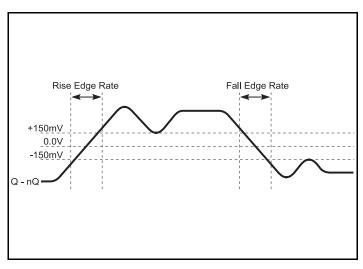
Differential Measurement Points for Rise/Fall Edge Rate
