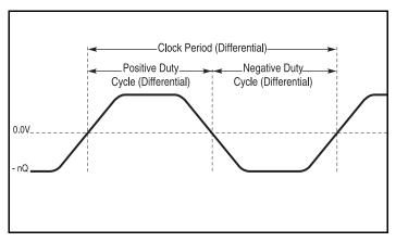
**Differential Measurement Points for Duty Cycle/Period**
