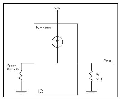
Figure 5. HCSL Driver Circuit and Termination
