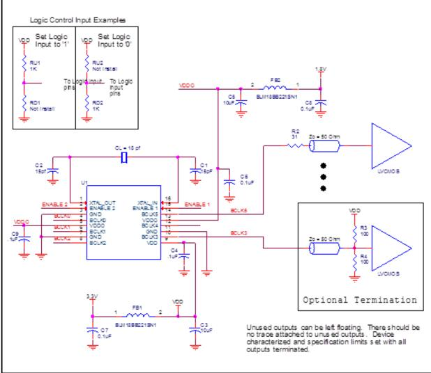
Figure 4. Schematic of Recommended Layout
