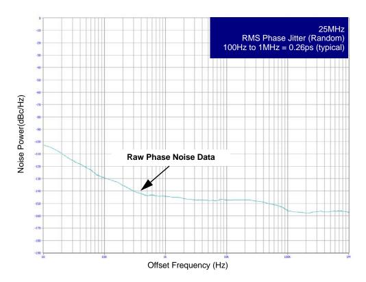
Typical Phase Noise at 25MHz (2.5V Core/2.5V Output)
