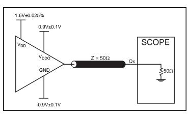
2.5V Core/1.8V LVCMOS Output Load AC Test Circuit
